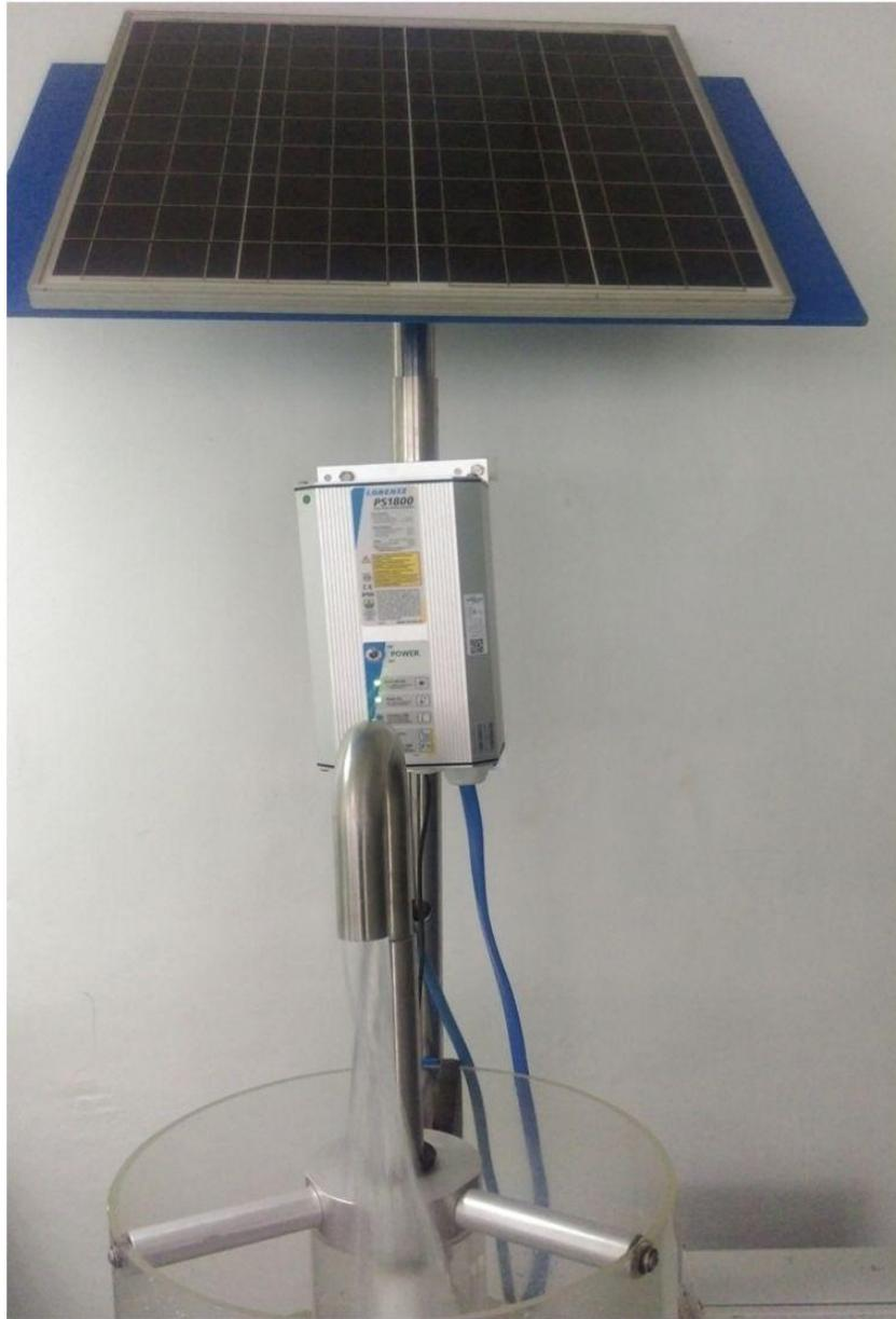
Solar water pumping system with flow meter and controller
