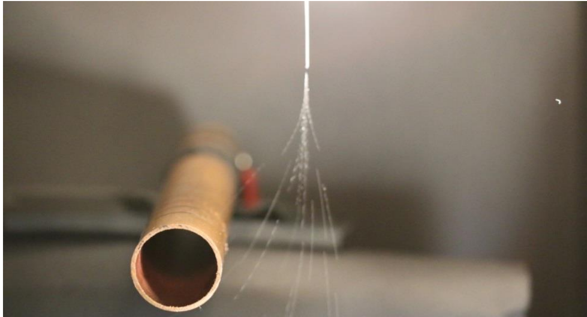
Figure 4.2: Attraction of Droplets to Tube
