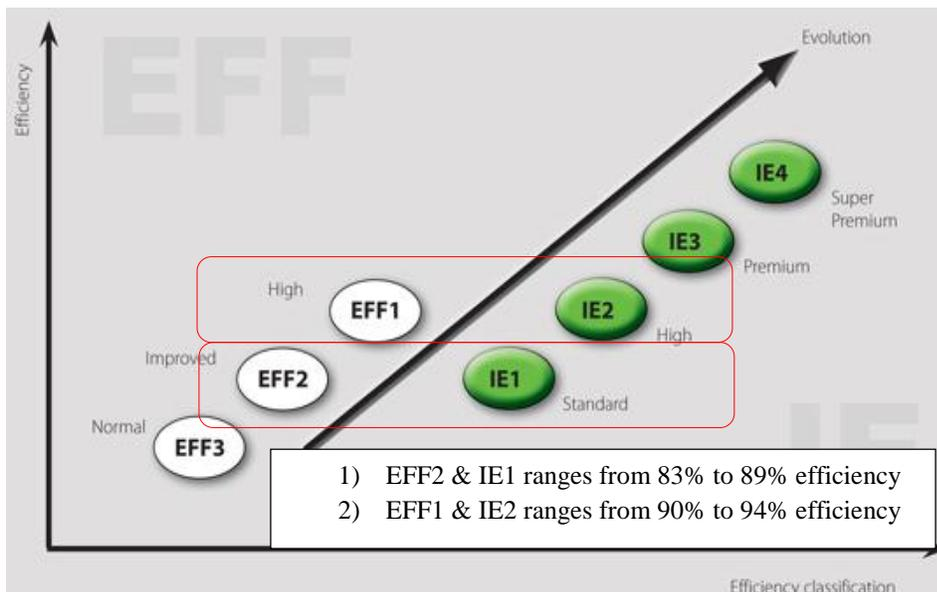
**Figure 2.5: World standard motor efficiency classification**
