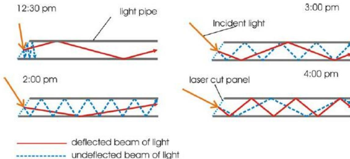
**Figure 2.11: transmission of light through horizontal pipes for the deflected and undeflected beam of light at different times of the day**
