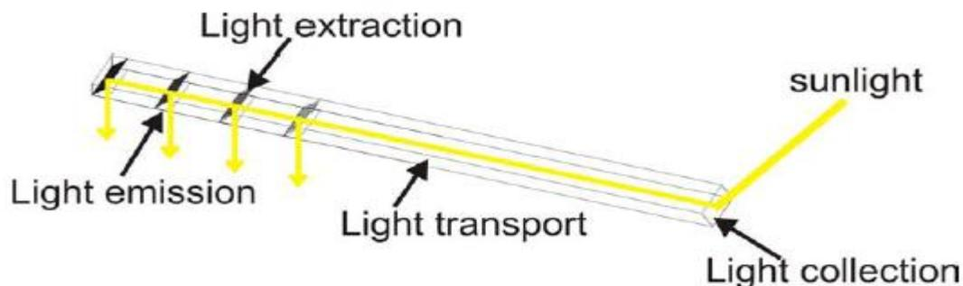
**Figure 2.7: Light piping system diagram**
