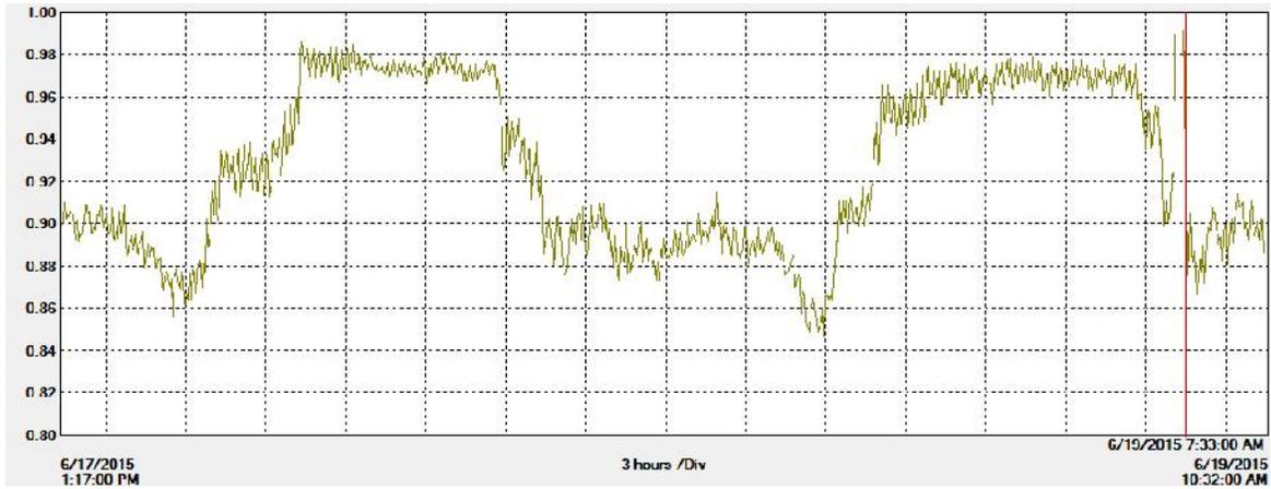
**Figure 4.20: Logged power factor for Lift 1**
