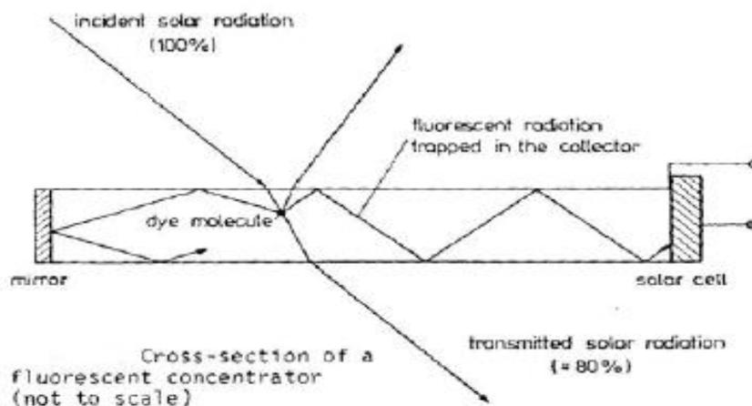
**Fig 2.10: Cross-section of a fluorescent concentrator.**
