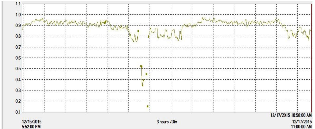
**Figure 4.21: Logged Power Factor for Lift 2.**
