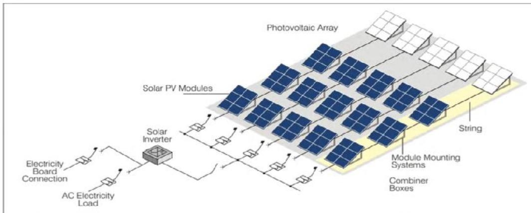
**Fig 2.2: Typical Solar PV System Architecture**
