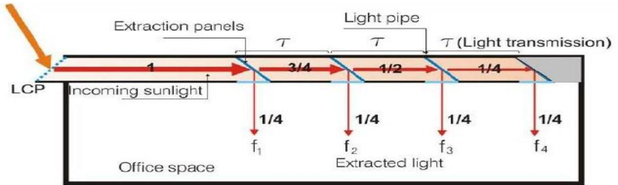
**Fig 2.12: Light extraction in the light pipes**
