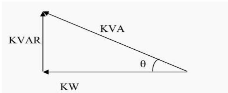
**Figure 4.18 (b): Power Factor Vector diagram**
