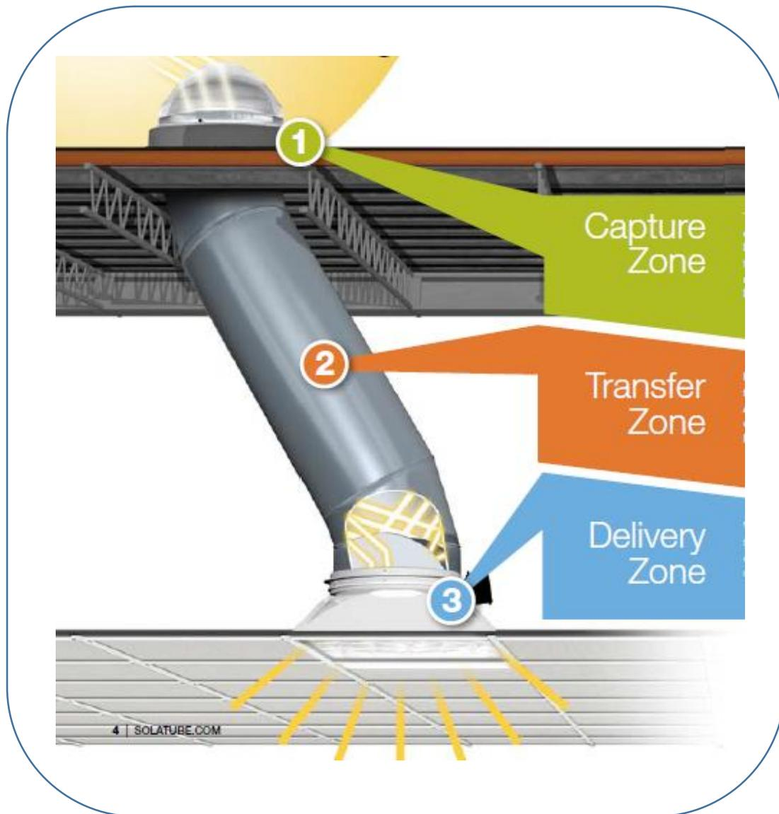
**Fig 2.8: Typical Light-pipe system**
