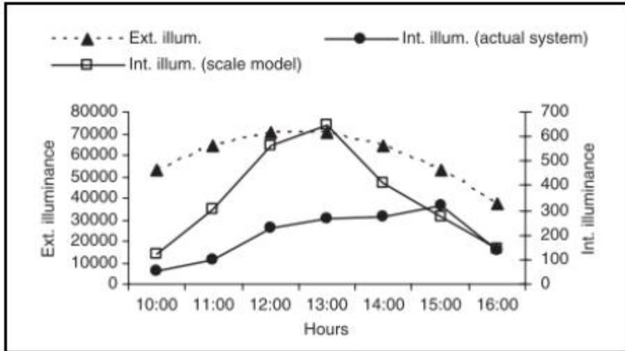
**Figure 4.10: Test performance for a 560mm Diameter, 25M Length light pipe**
