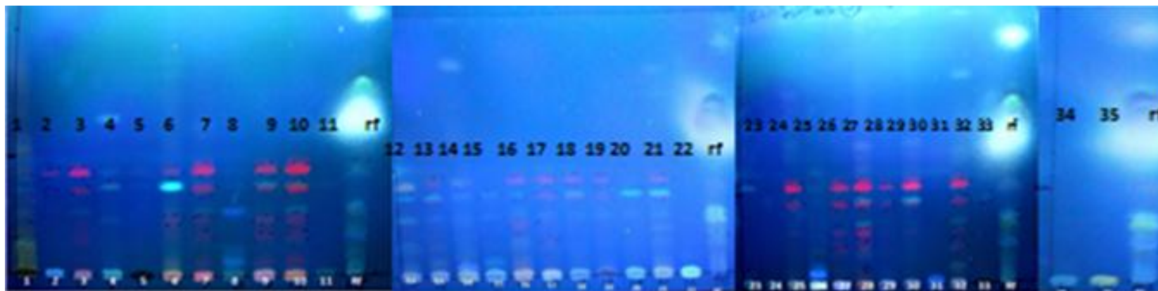
Figure 4.7 TLC chromatogram showing possible Essential oils as seen under UV. Lane labeled 1-35 represents the different extracts as described in Table 4.1 with the label rf representing the reference standard anethole, carvone, 1, 8-cineol (eucalyptol), eugenol, menthol and thymol for the phytochemical class.
