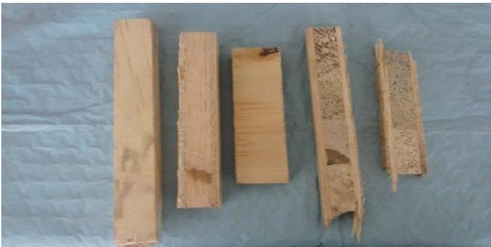
Figure 3.1.4: Blockboard sample
