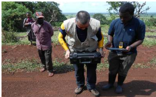
Height correction measurements for the PGIS-128 gamma spectrometer at the base of Mrima Hill.
