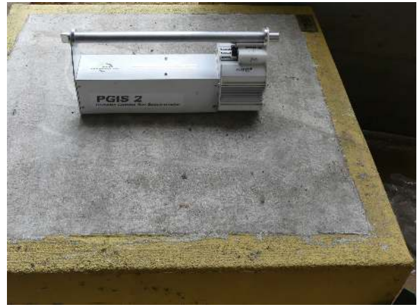
PGIS-21 detector on a 1 \times 1 \times 0.3 m thorium calibration pad.
