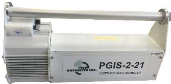
PGIS-21 consisting of a 0.33 l. NaI (Tl) detector.
