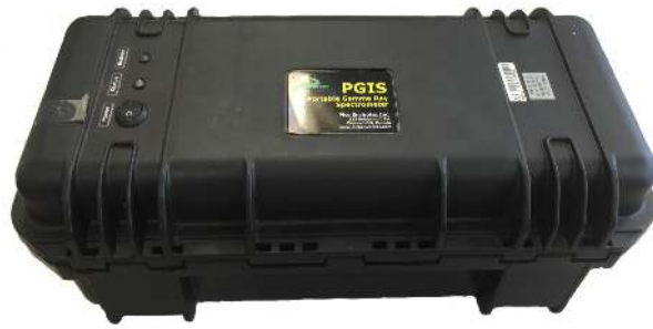
PGIS-128 consisting of a 2.0 l. NaI (Tl) detector.
