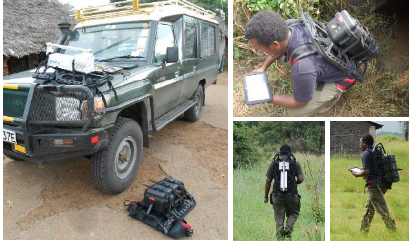
Motor vehicle used for in-situ vehicular radiometric measurements. Detector was laid horizontally inside the vehicle's floor.
