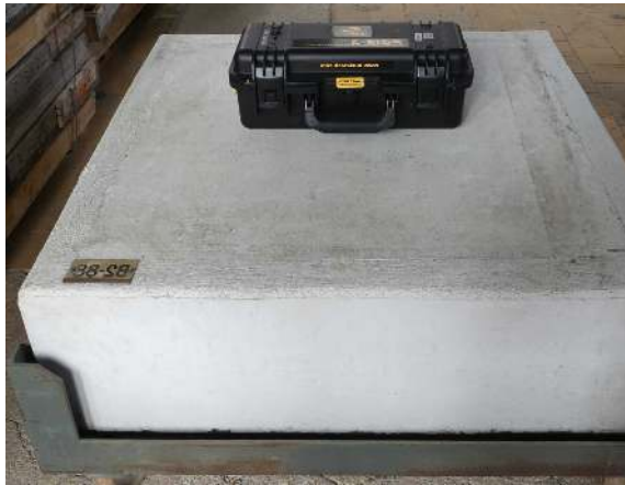
PGIS-128 detector on a 1 \times 1 \times 0.3 m background calibration pad.
