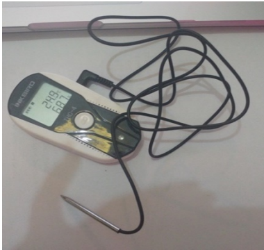
Fig 3-6: INKBIRD Data Logger used for collecting the temperature and relative humidity of View Park Towers. Source: Author
