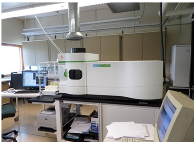
Figure 3.6: PerkinElmer 8300 bench top ICP-OES for sample analysis at MTT Finland.
