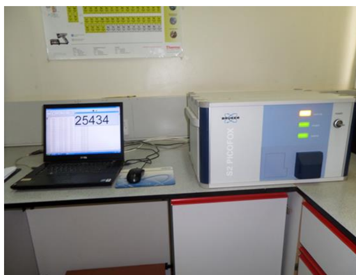
Figure 3.4: Bench top TXRF for sample analysis at ICRAF.
