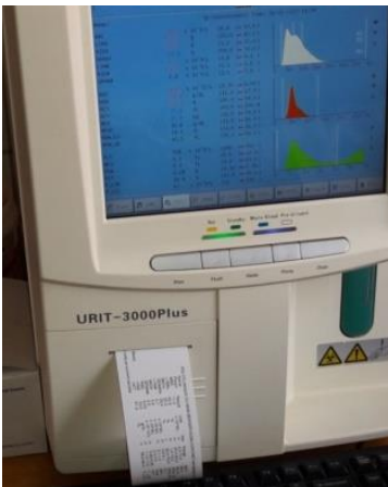
Figure 8 : Automated haematology analyser used for analysing EDTA-K2 blood samples
