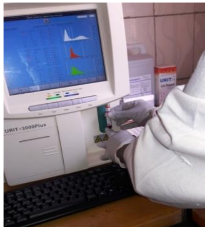
Figure 8 : Automated haematology analyser used for analysing EDTA-K2 blood samples
