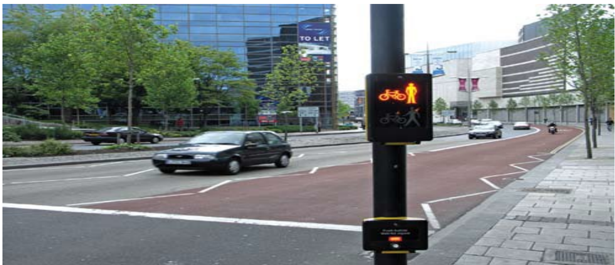
Figure 6–3: Near-side pedestrian signal with confirmation light in Bristol, UK
