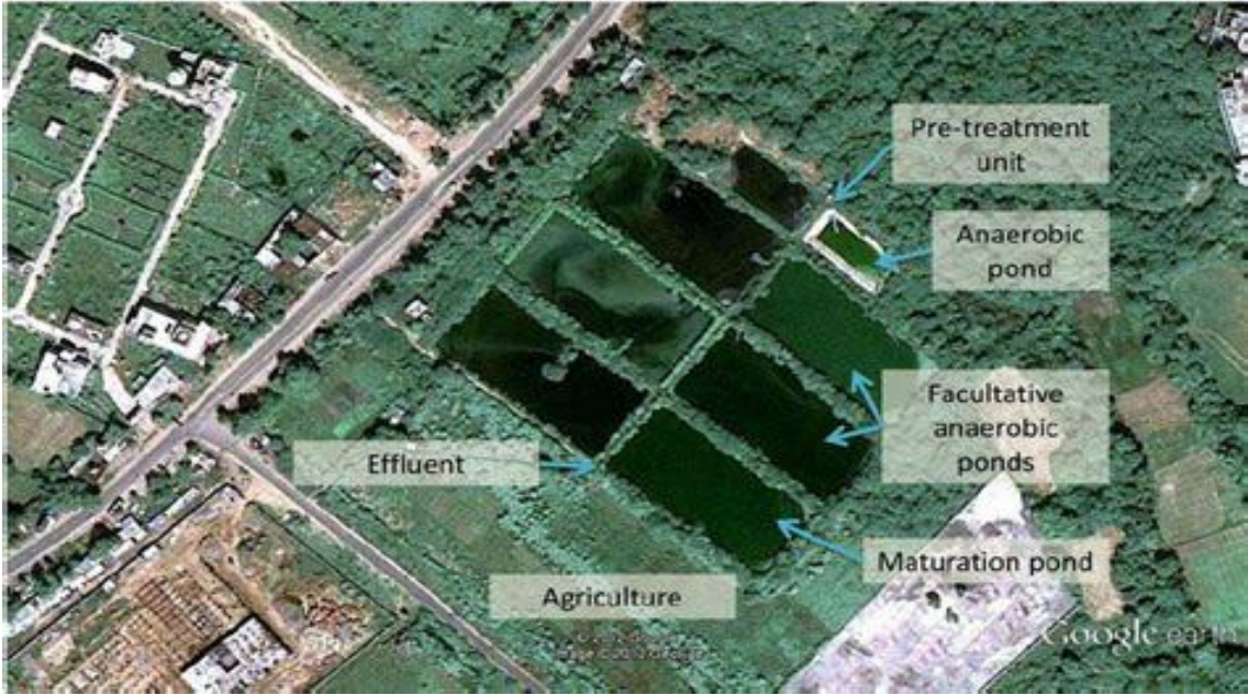
Figure 4: Schematic flow chart of waste stabilization ponds of Mathura III in India, Source: Amerasinghe et al, 2013
