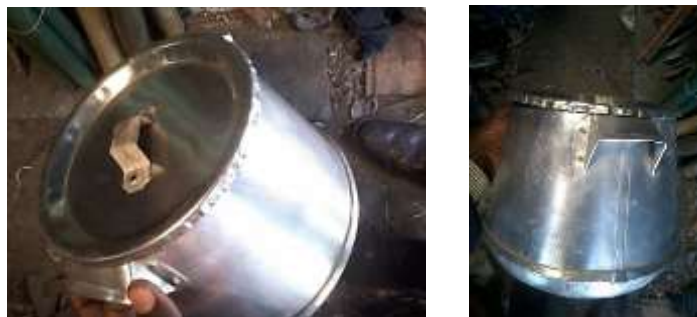
Figure 37: Boiling pot with twisted edges on the lid
