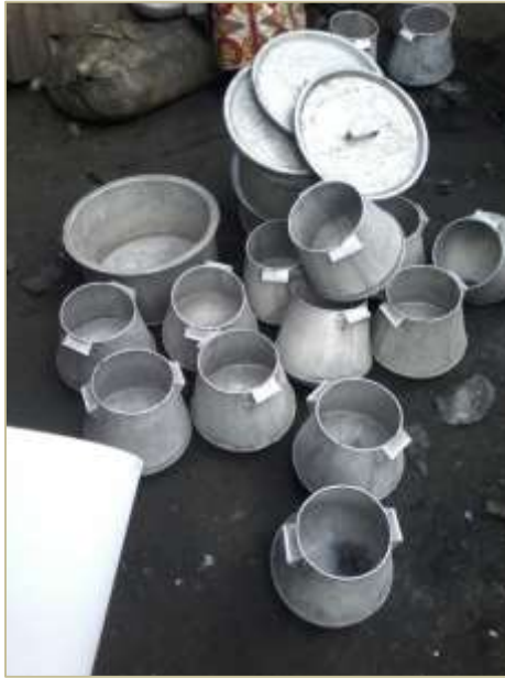
Figure 68: Fabricated sheet aluminium boiling pots at the cleaning stage at Kamukunji
