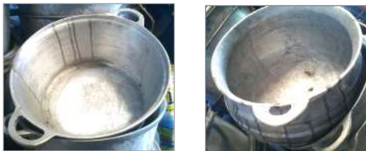
Figure 14: Permanent streaks of acid stain marks on cookware
