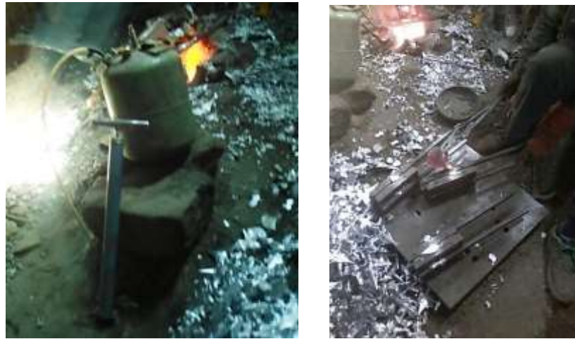
Figure 26: Images showing pressurized paraffin blow torch used as a furnace catalyst
