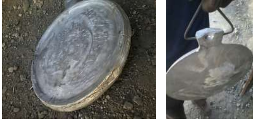
Figure 29: Flat disc frying pan with inconsistent surface
