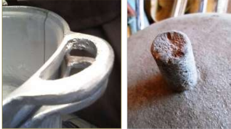
Figure 31: Resulting cast from defective models showing rough cookware handles
