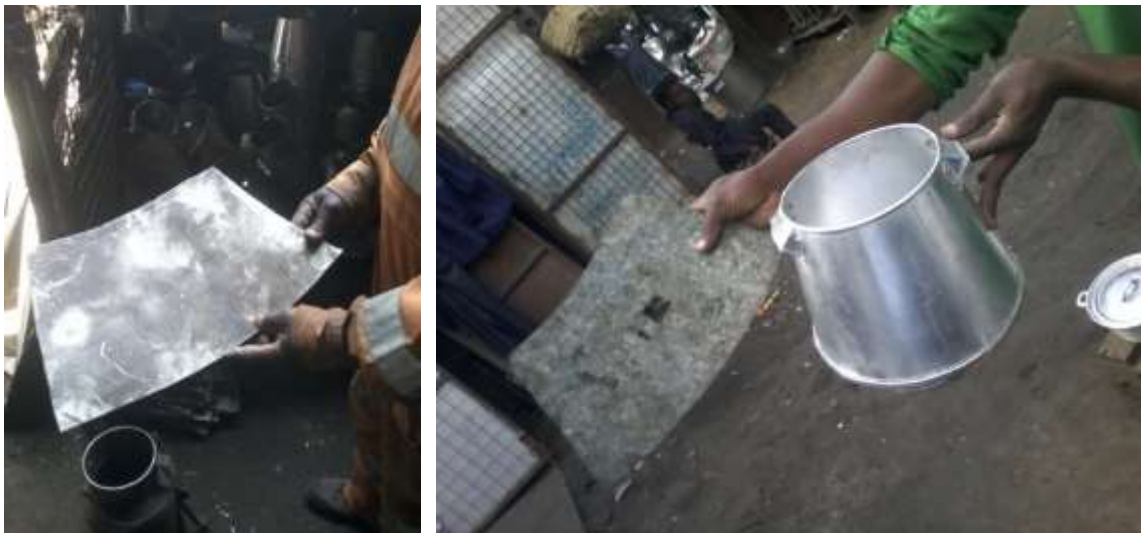
Figure 7: Comparison of aluminium and galvanized steel template
