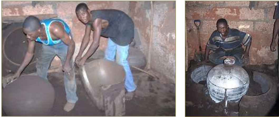
Figure 3: Cast pot broken away from sand mold Source: https://benistoves.wordpress.com/
