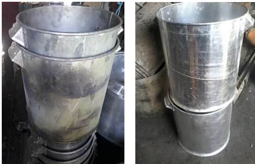
Figure 23: Comparison of recycled sheet aluminium and standard sheet aluminium.
