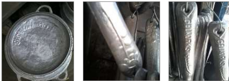
Figure 39: Flaws on branding elements and floral designs
