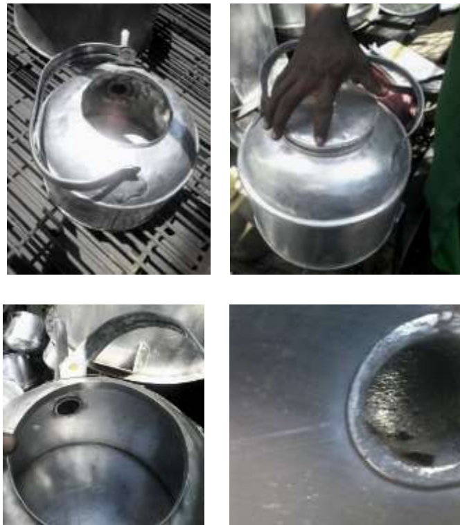
Figure 35: Aluminium kettle with inconsistent lid dimensions and joining of the spout
