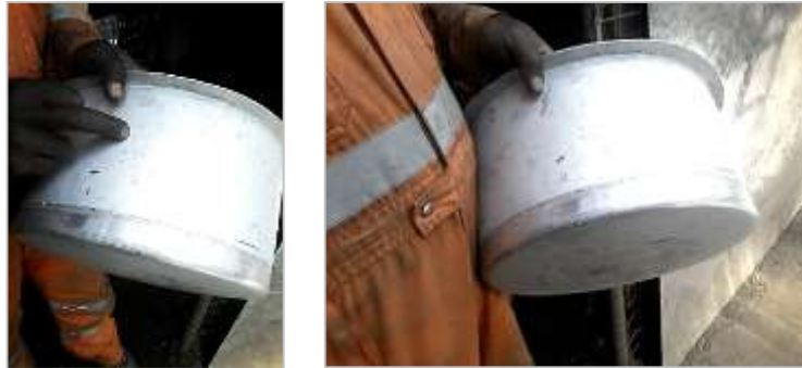
Figure 20: Cooking basin made from recycled milk can
