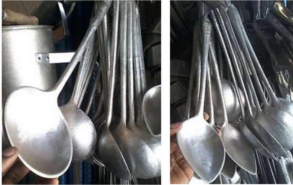
Figure 40: Sand cast spoons and servers with decorated bands on handles
