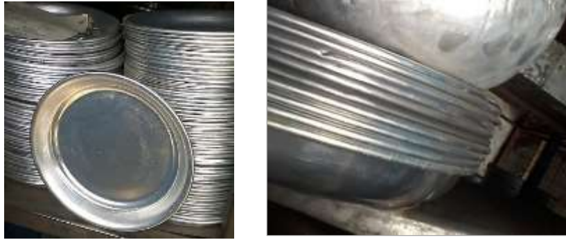
Figure 34: Plates and tray derived from sheet metal spinning
