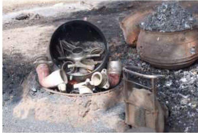
Figure 1: A cupola filled with scrap aluminium from vehicle parts Source: https://benistoves.wordpress.com/
