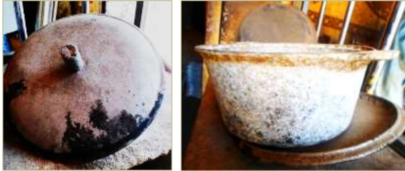
Figure 18: Cookware model used in making sand casting moulds showing corrosion marks
