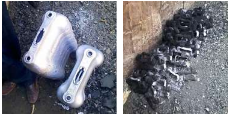
Figure 62: Cast weighing scale base and sections
