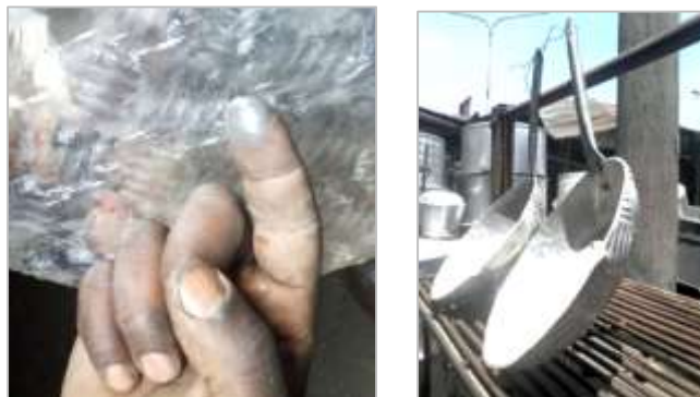
Figure 19: Rubbing from textured aluminium sheet metal used in making shallow frying pans
