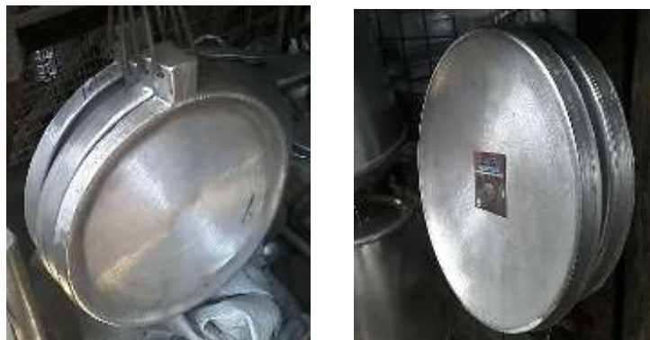
Figure 32: Successful die cast flat disc frying pans
