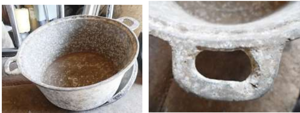
Figure 30: Casting model with detail of flaws in geometry
