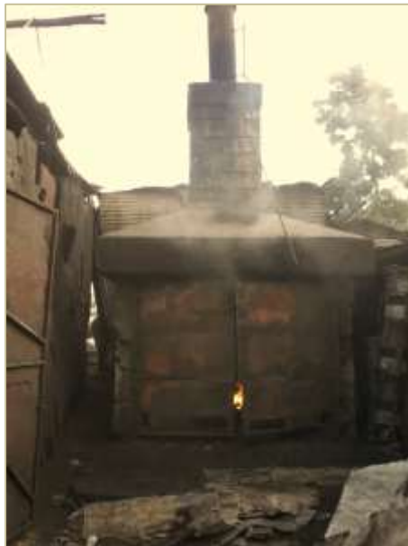
Figure 69: Furnace for annealing metal at Kamukunji
