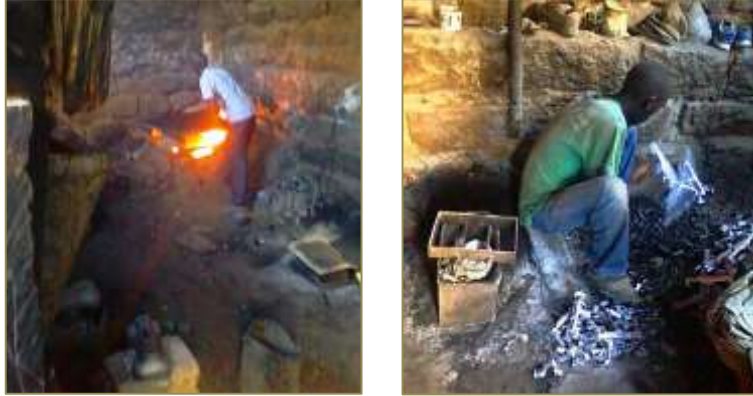
Figure 61: Sand casting workshop for parts of weighing scales
