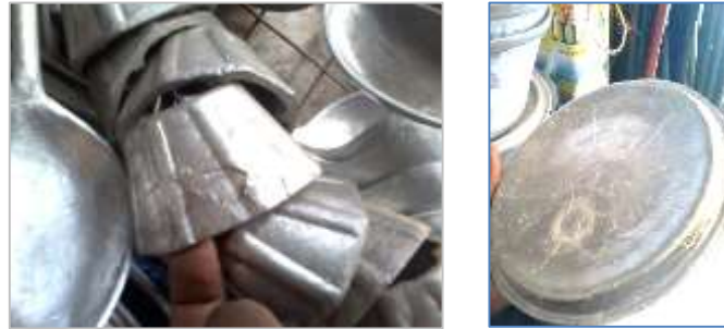
Figure 12: Maize shredder with cracked surface and boiling pot lid showing and fissures
