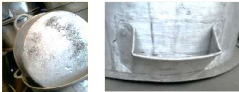
Figure 13: Cookware showing pores and repaired tearings
