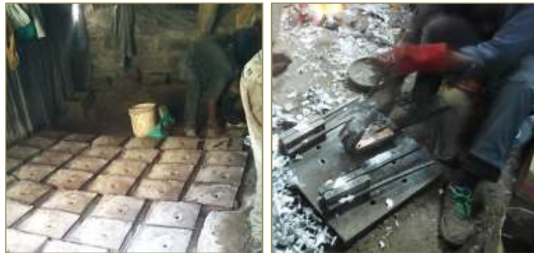
Figure 10: Sand casting molds and die casting moulds. Source: Author
