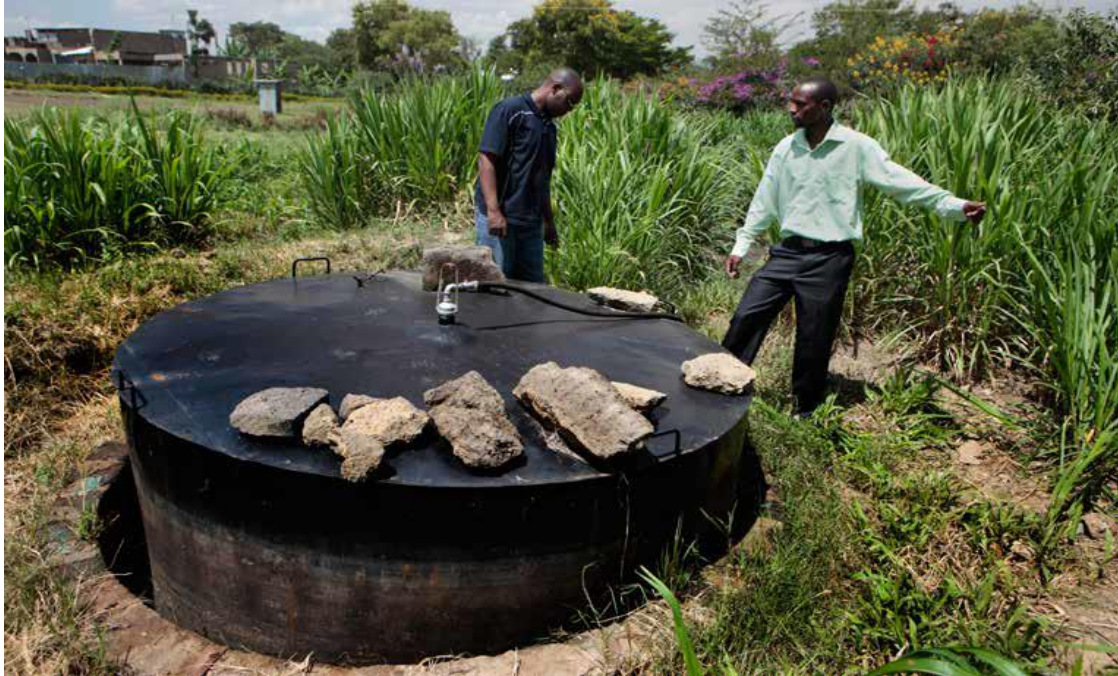
Plate 71: Biogas plant- source of Methane for lighting and cooking (Adopted from Carabine et al., 2014)
