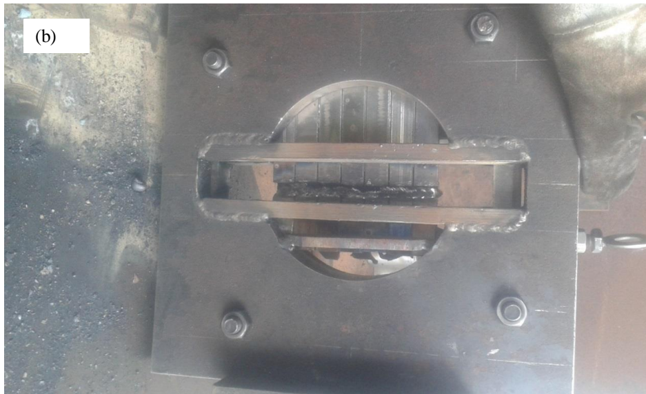
Figure 3.5: (a) Bottom plate of welding fixture and (b) welded bars clamped in fixture
