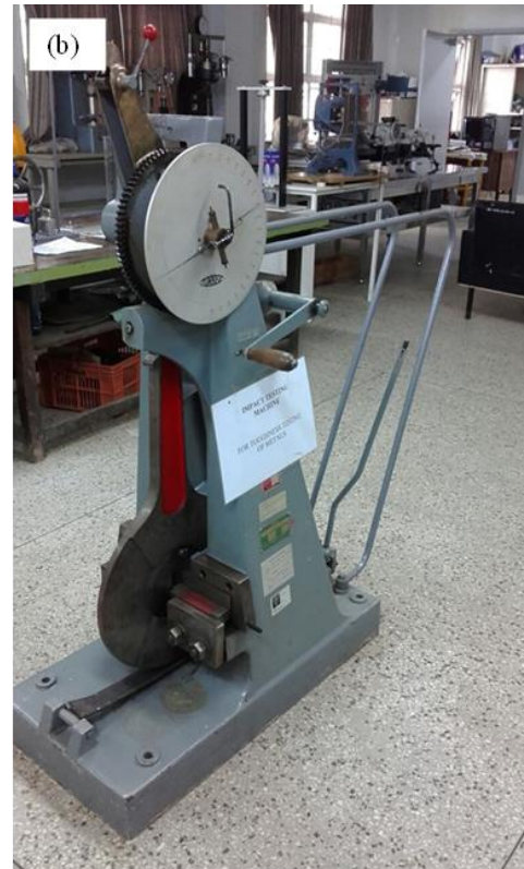
Figure 3.11: (a) INSTRON universal hydraulic tensile testing machine and (b) Charpy V-Notch impact tester
