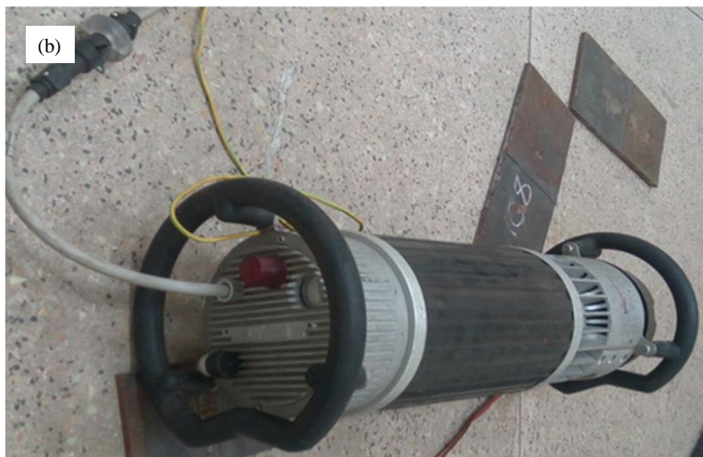
Figure 3.8: (a) Karl Deutsch Digital Echograph 1090 used in ultrasonic inspection and (b) Portable X-Ray tube YXLON Y SMART300HP used in radiographic inspection
