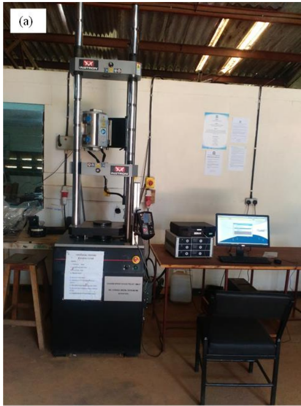
Figure 3.11: (a) INSTRON universal hydraulic tensile testing machine and (b) Charpy V-Notch impact tester
