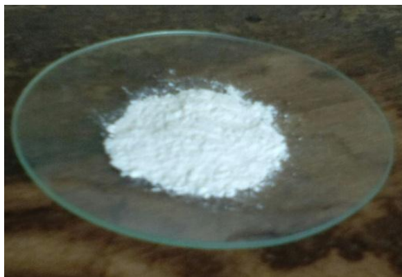
Fig. 4.2: 150 \mu m mesh- size composite powder after annealing and pulverization
