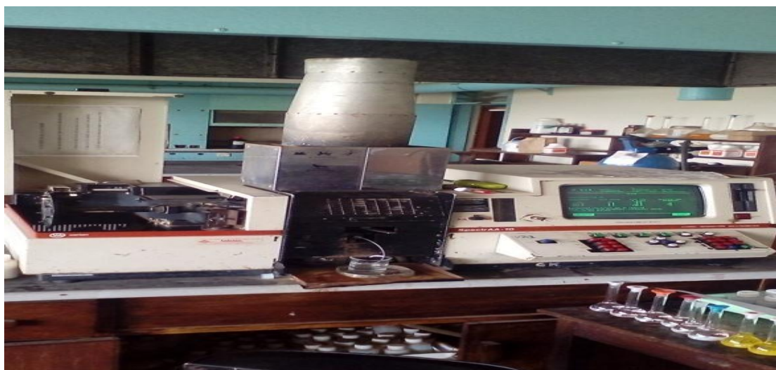
Figure 3.1: A Varian SpectrAA-10 AAS Spectrophotometer used for aqueous heavy metal analysis at the Geochemistry Labs, Ministry of Mines (G.o.K), Nairobi.
