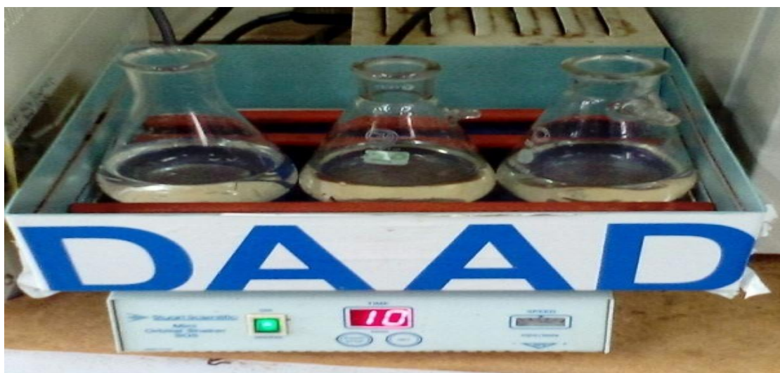
Fig 3.2: Batch adsorption experimental set-up using an Orbital Shaker at the Pesticides and POPs Lab, Chemistry Dept. CBPS, UoN.
