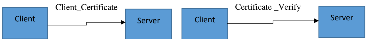
SSL phase 2 - client response to server.
