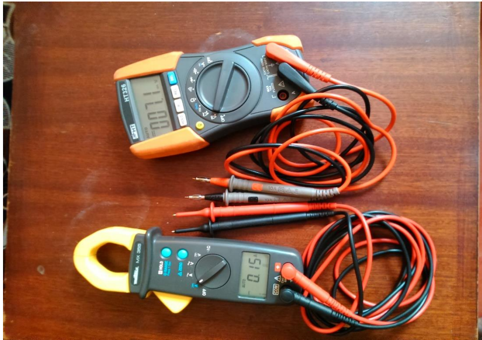
Figure 4.10: The digital multimeters for calibrating the voltage and current scales of the BMS
