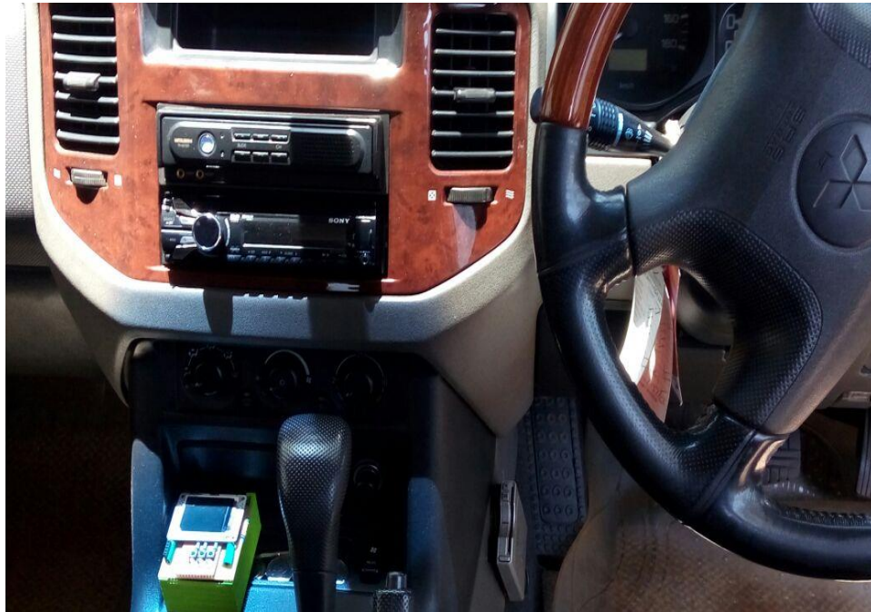
Figure 4.15: The battery monitoring system display, the green box, in the 250 Hp engine car
