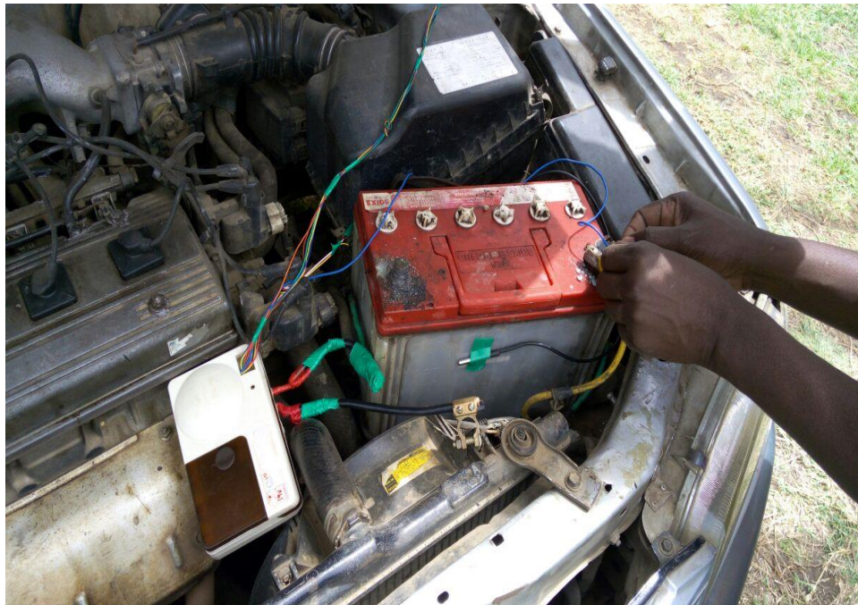
Figure 4.14: The battery monitoring system installed in the 115 Hp engine car
