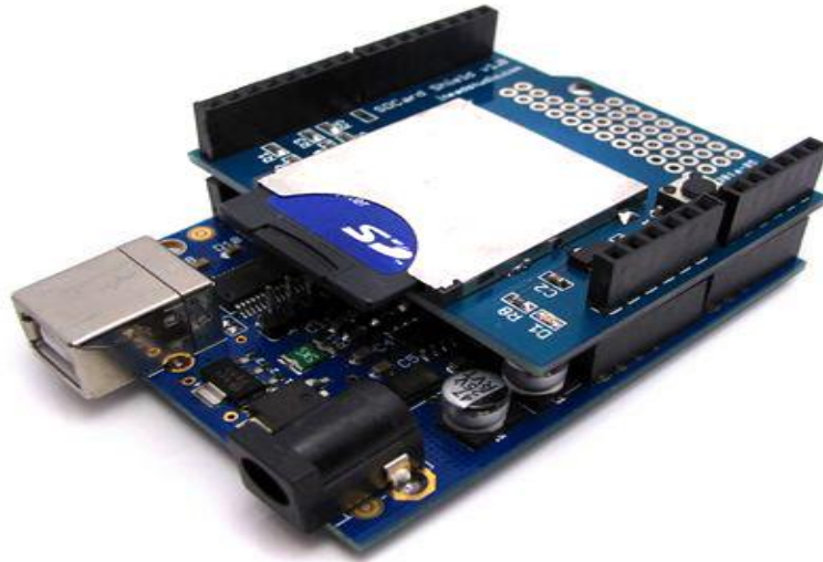
Figure 4.8: The data logger bearing the SD card mounted on the Arduino Uno R3 board
