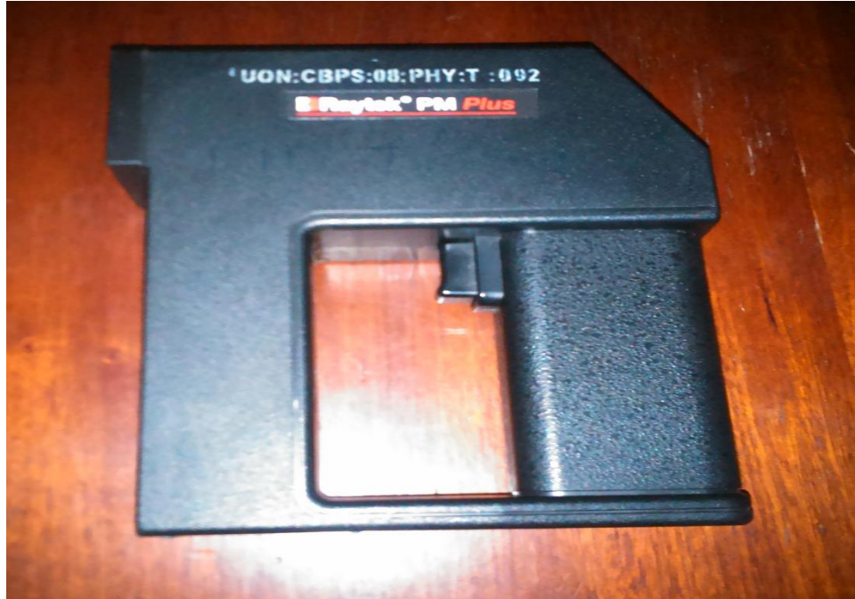
Figure 4.11: The IR Raytek thermometer for calibrating the temperature scale of the BMS
