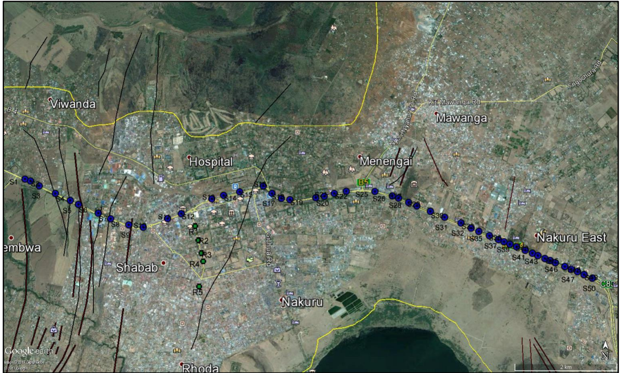
Figure 4.2 Google earth image of the survey area. The ReMi points are plotted as blue circles
