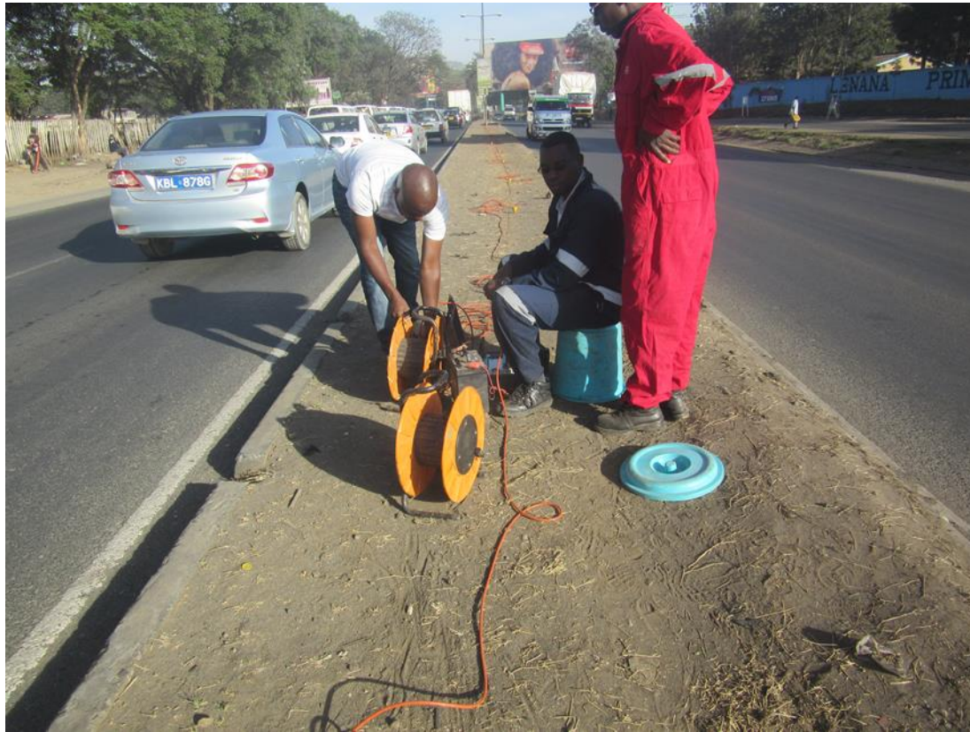
Figure 3.4 A photo taken during the field exercise showing the field layout of the linear ReMi array
