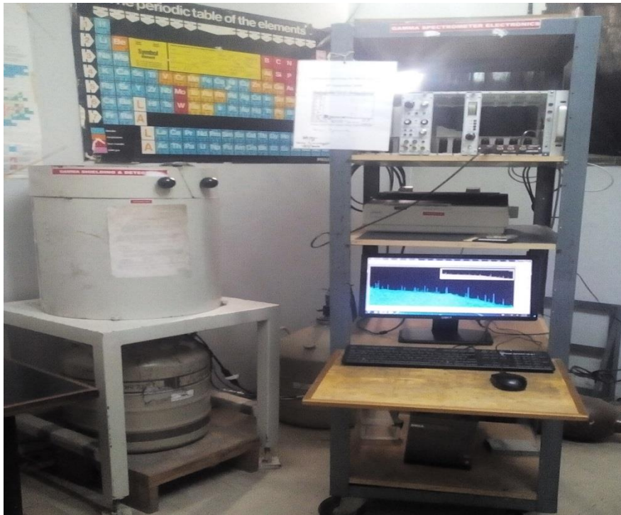
Figure 3.3: A set up of HPGe gamma spectroscopy at the Institute of Nuclear Science & technology
