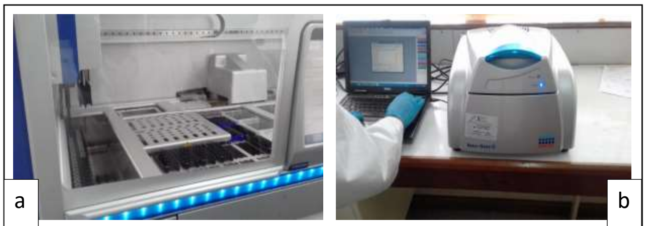
Figure 2: DNA extraction and PCR amplification Equipment. (a) QIASymphony for automatic DNA extraction (b) Rotor-Gene Q (Qiagen, Germany)
