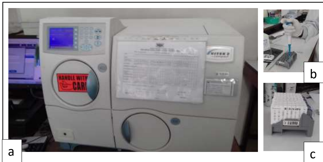
Figure 1: VITEK ® 2 (a) Image of machine (b) Dilution of cultured pathogens (c) ID and AST cassettes
