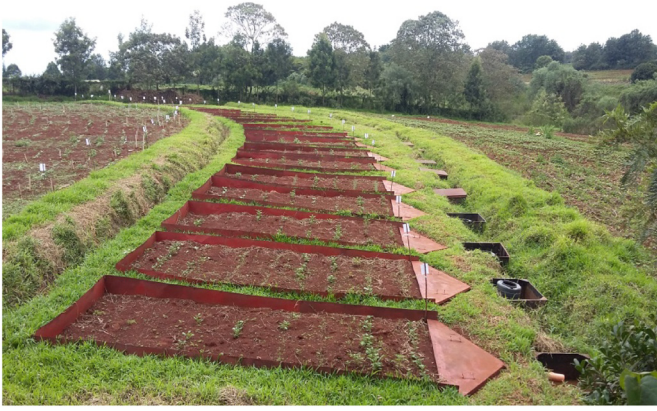
Fig. 1. Runoff plots installed at right angle to the contours and parallel to the slope.
