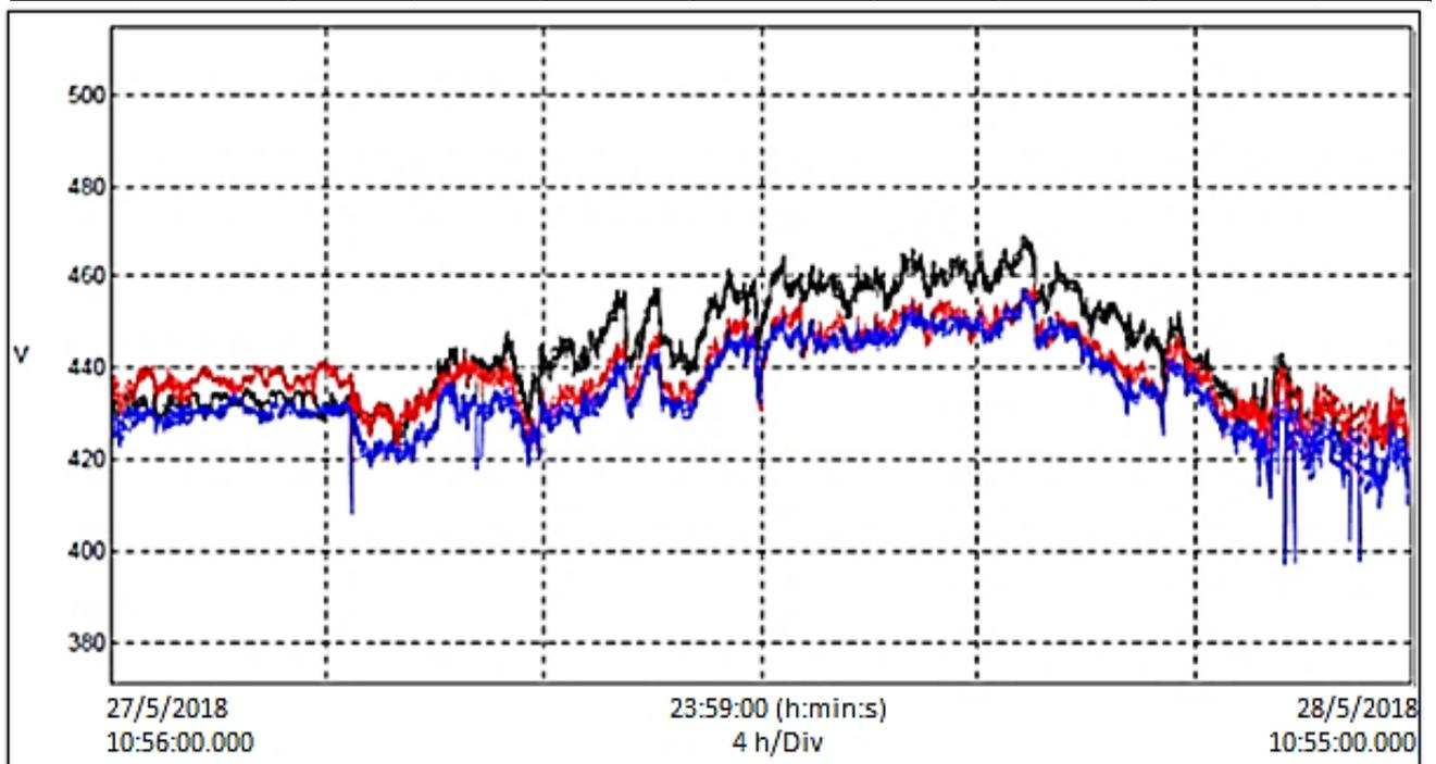
Figure 4. 5: Variations of utility energy supply voltage
