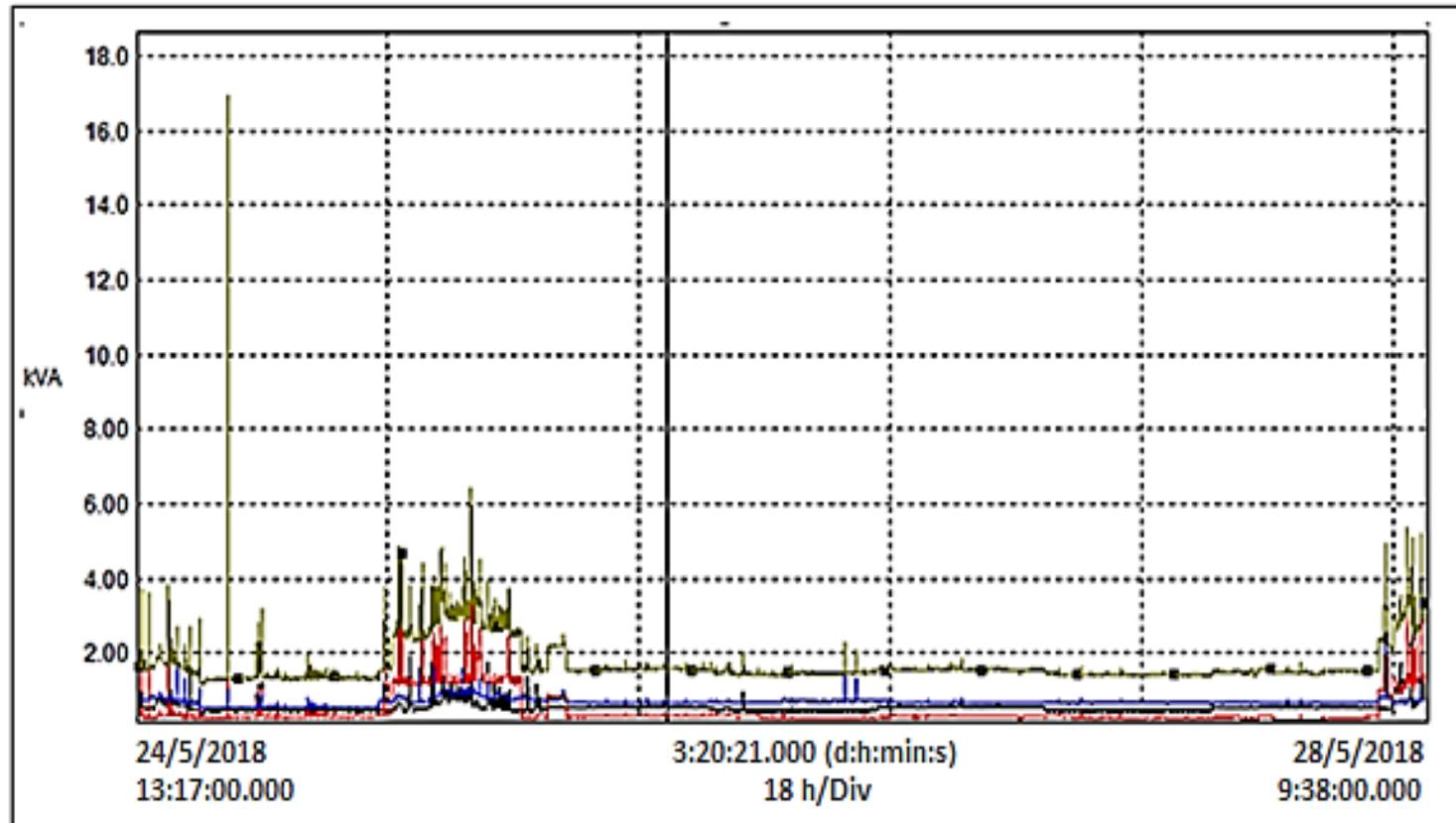
Figure 4. 6:Energy demand load profile for the NCCRC
