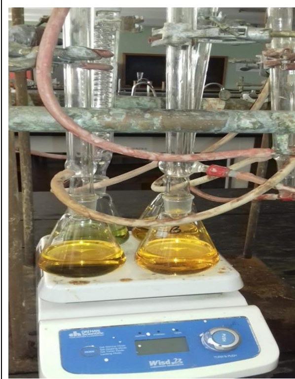
Plate 2.9: Pictorial showing Determination of COD of wastewater
