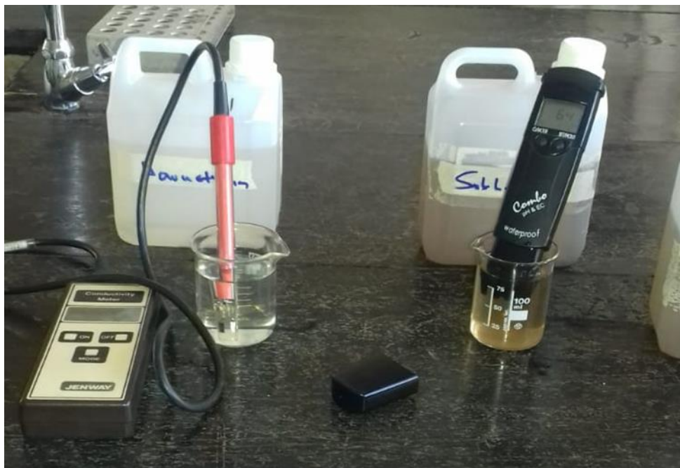
Plate 3.2: Pictorial showing process in determination of EC
