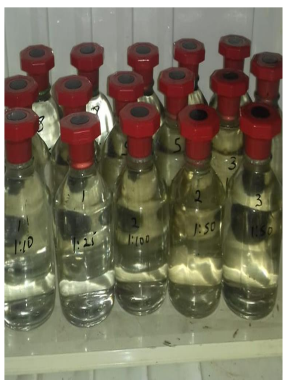
Plate 2.10: Pictorial showing Determination of BOD of wastewater
