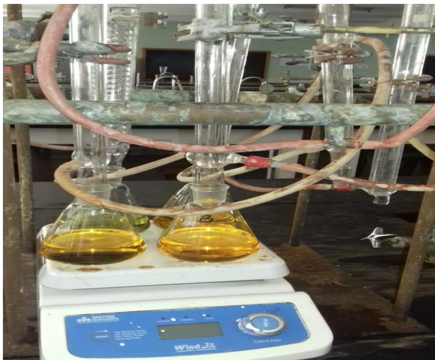
Plate 3.3: Pictorial showing process in determination of COD of wastewater
