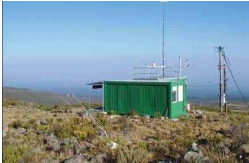
Fig 3.4 Mount Kenya Global Atmospheric Watch (GAW) station a Meteorological station collecting Surface Ozone data
