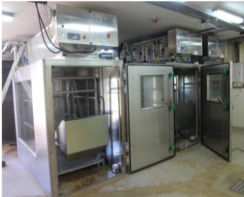
Plate 3-3: Methane animal respiratory chamber
