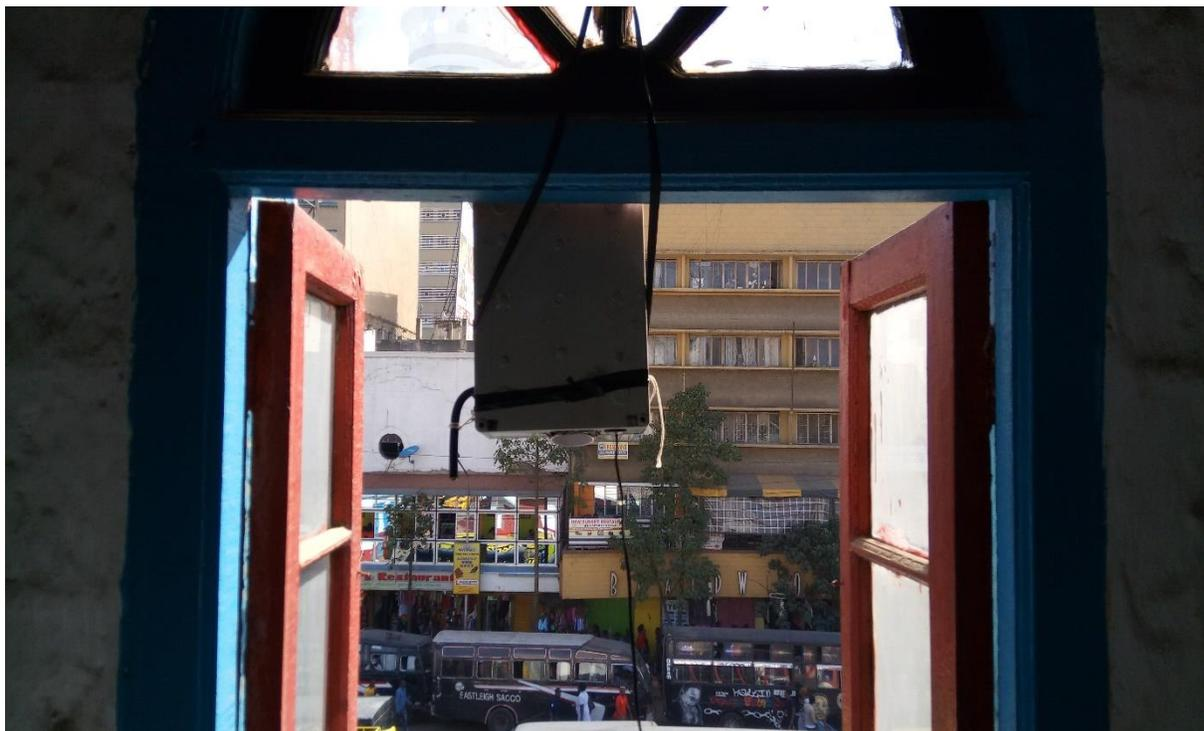
**Figure 3. 5:Shows one of the OPC-N2 deployed at the urban roadside site in Nairobi.**
