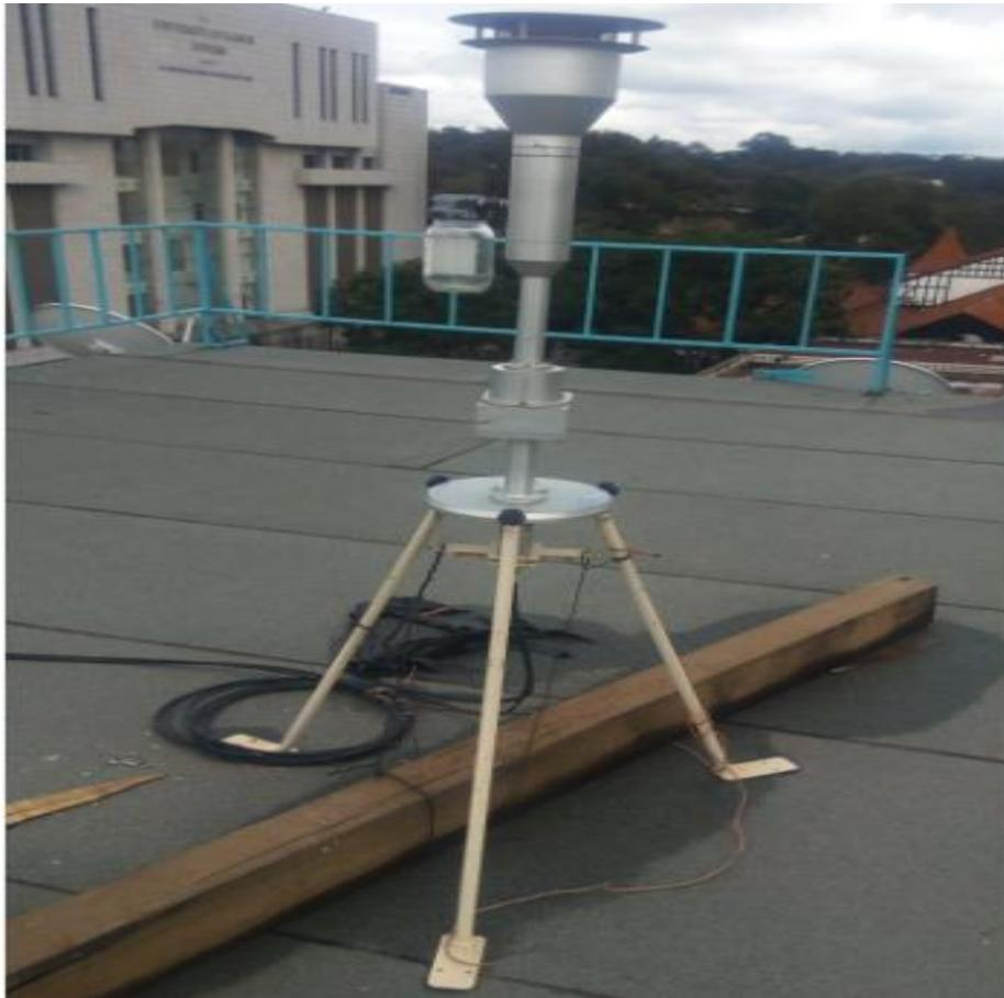
Figure 3. 3: Andersen dichotomous air sampler deployed on the roof of the American Wing Site at the UoN.
