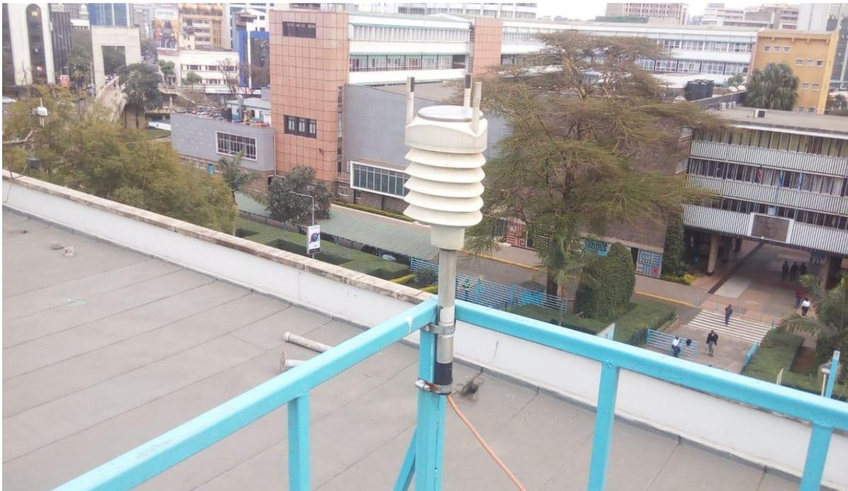
**Figure 3. 4: Vaissala weather instrument deployed at the American Wing Site.**
