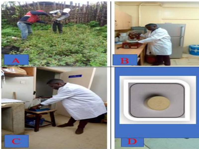
Figure 3.3: Photos summarizing the research procedure (A-Sampling of the Soil and Spider plants, B-Pulverization of the samples, C-Pellet preparation by the use of the hydraulic pellet press and D- Pellet ready for EDXRF analysis)
