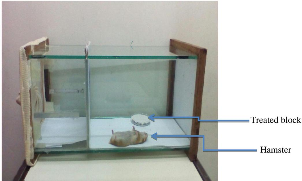
**Figure 3.1:** A plexi- glass tunnel layout used for sand fly and mosquito experiment
