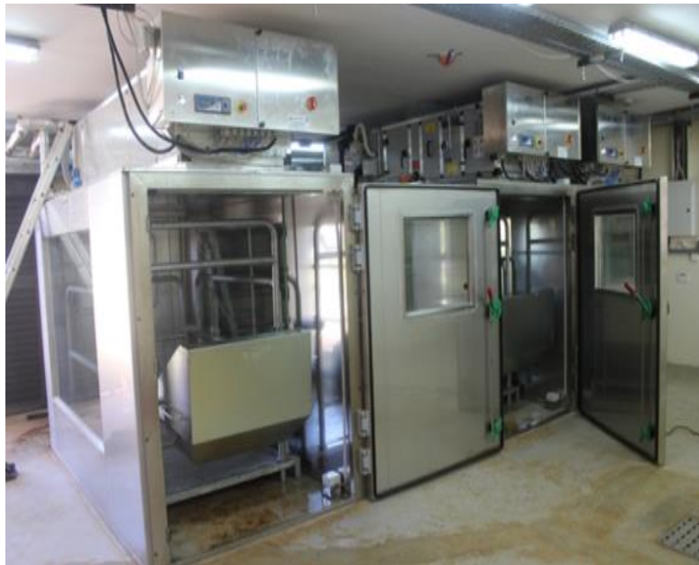
Plate 3-3: Methane animal respiratory chamber
