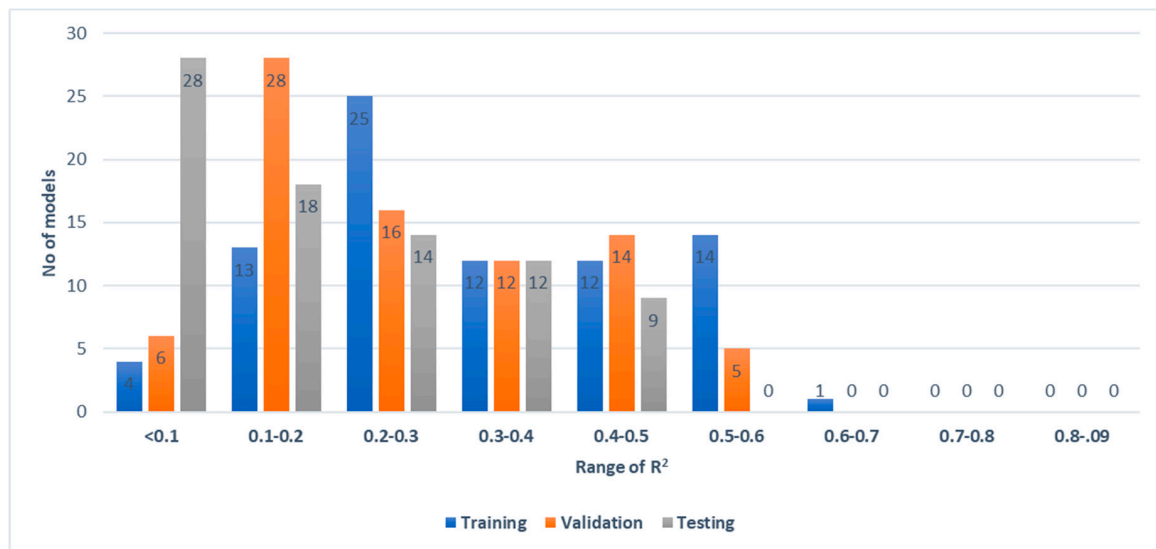
Figure 13. Distribution of non-selected models ANN performance on training, validation and testing. No model is noted to post an R 2 of at least 0.5 in testing.
