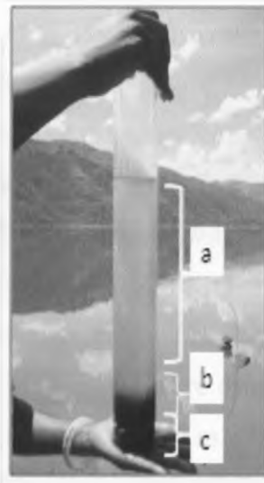
Plate 3.1: Gilson's corer showing the position of (a) the planktonic community, (b) the epipellic community in the water-mud interface and (c) sediment.
