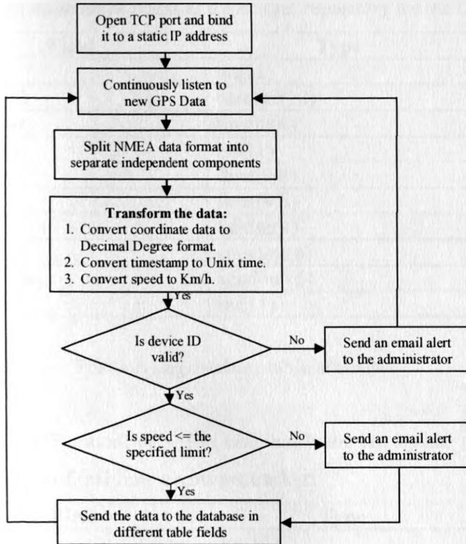
Figure 3.2: The flow chart for the GPS Data Receiver's functionality.
