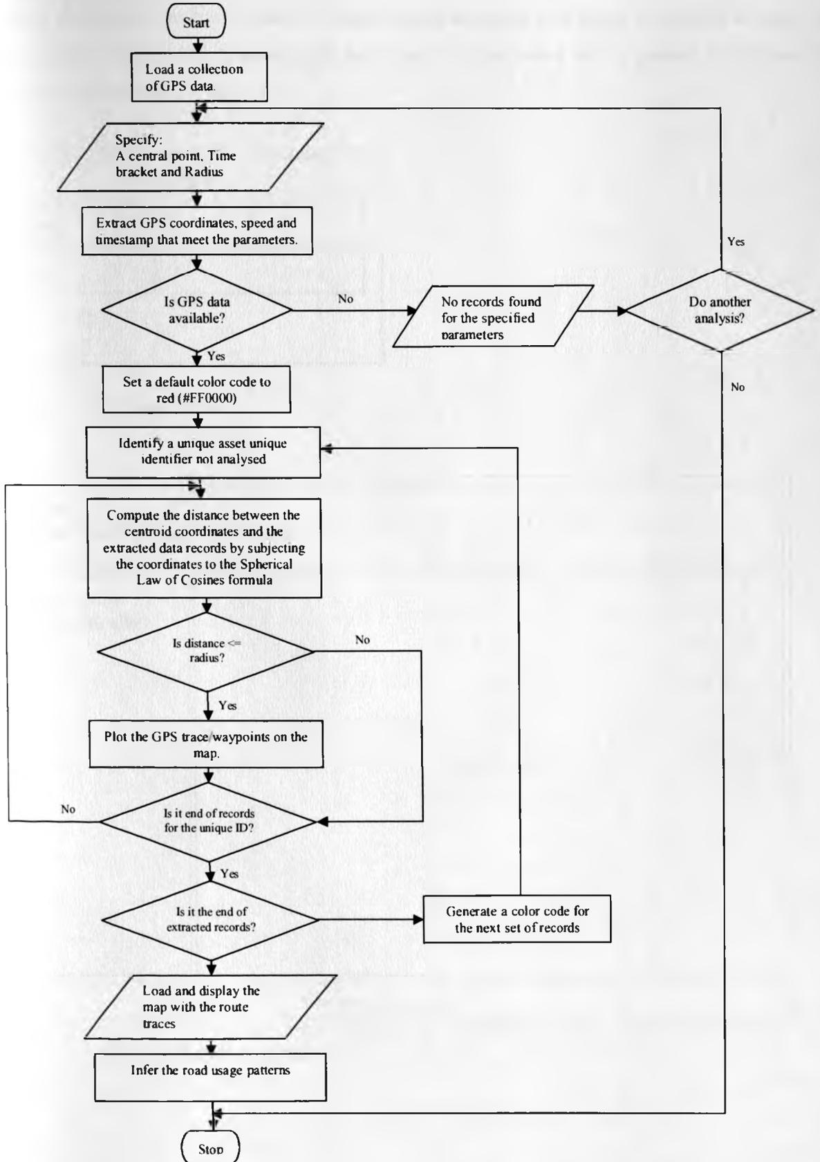
Figure 3.5: The flow chart for the road usage pattern algorithm.
