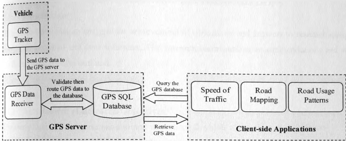
Figure 4.12: The model for the system.
