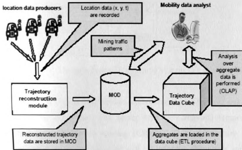
Figure 2.1: The Proposed framework for Mobility Data Warehousing and Mining (Marketos, 2009).
