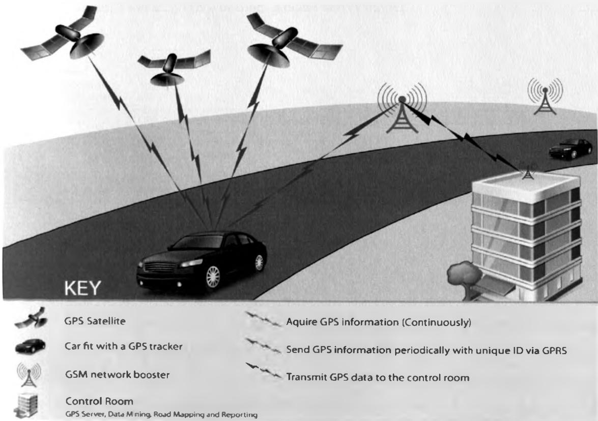
Figure 2.3: The concept of the system.
