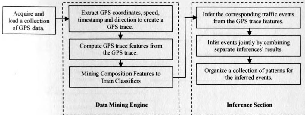
Figure 3.3: The flow chart for the data mining aspect.
