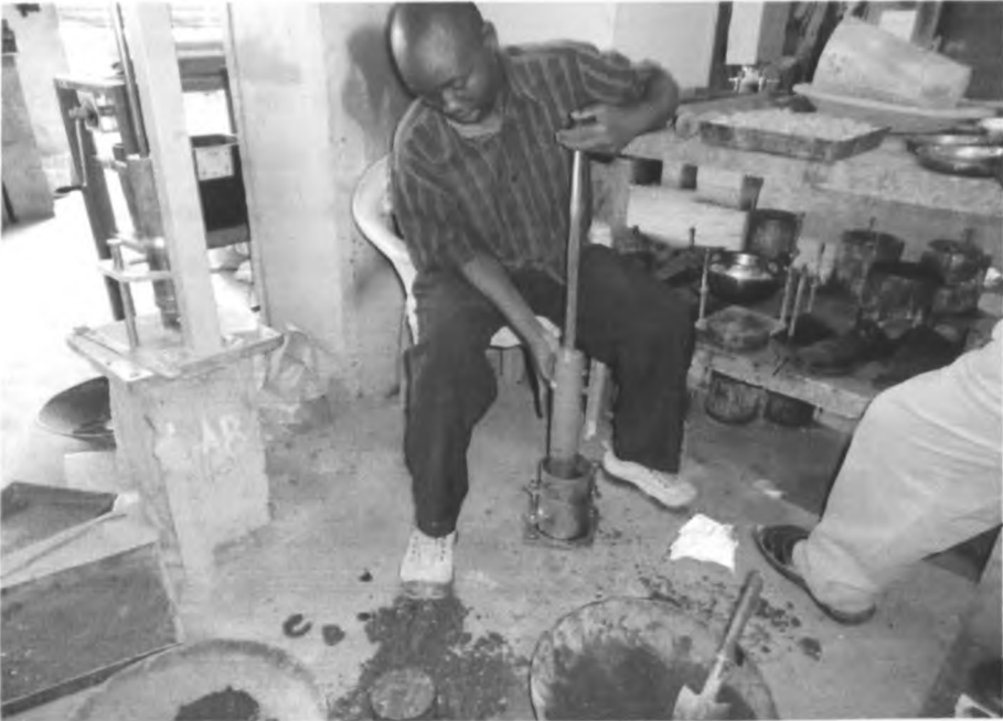
Plate 7: Compaction of soil sample-Proctor Test
