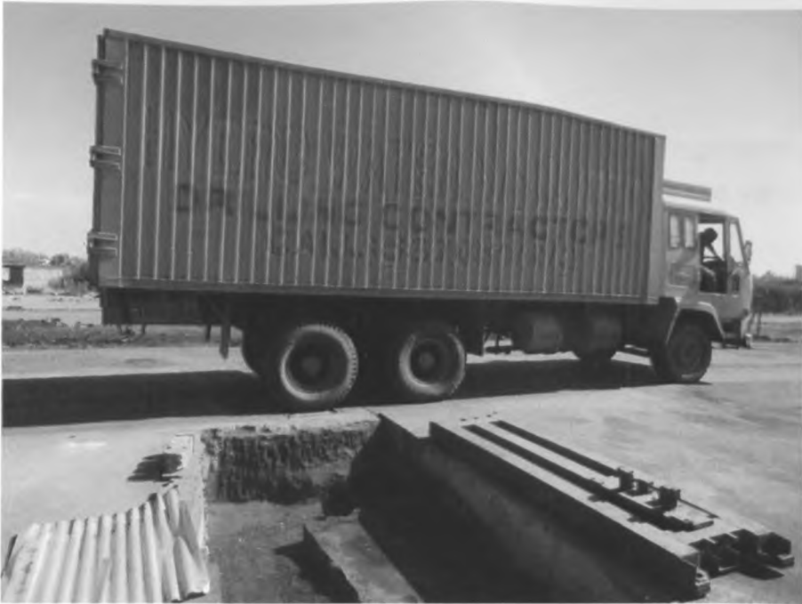
Plate 16: Weighing of a rigid body vehicle at the weighbridge
