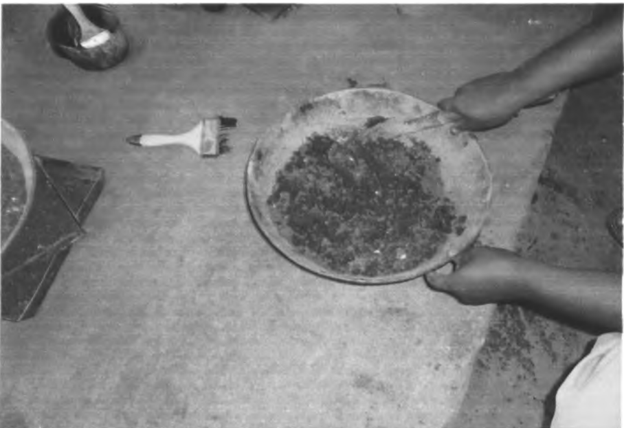
Plate 5: Mixing of soil sample with water-Proctor Test
