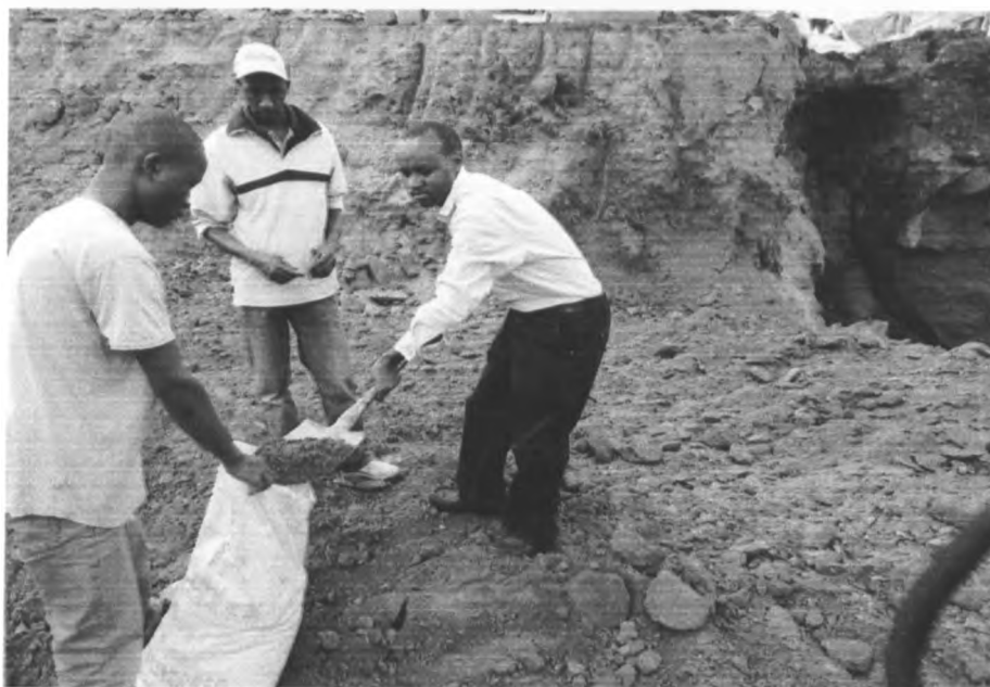
Plate 1: Material sampling @ the Pangani interchange
