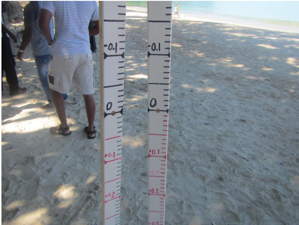
Figure 5: Survey wooden rod used for Emery Survey Method (Obare, 2016)
