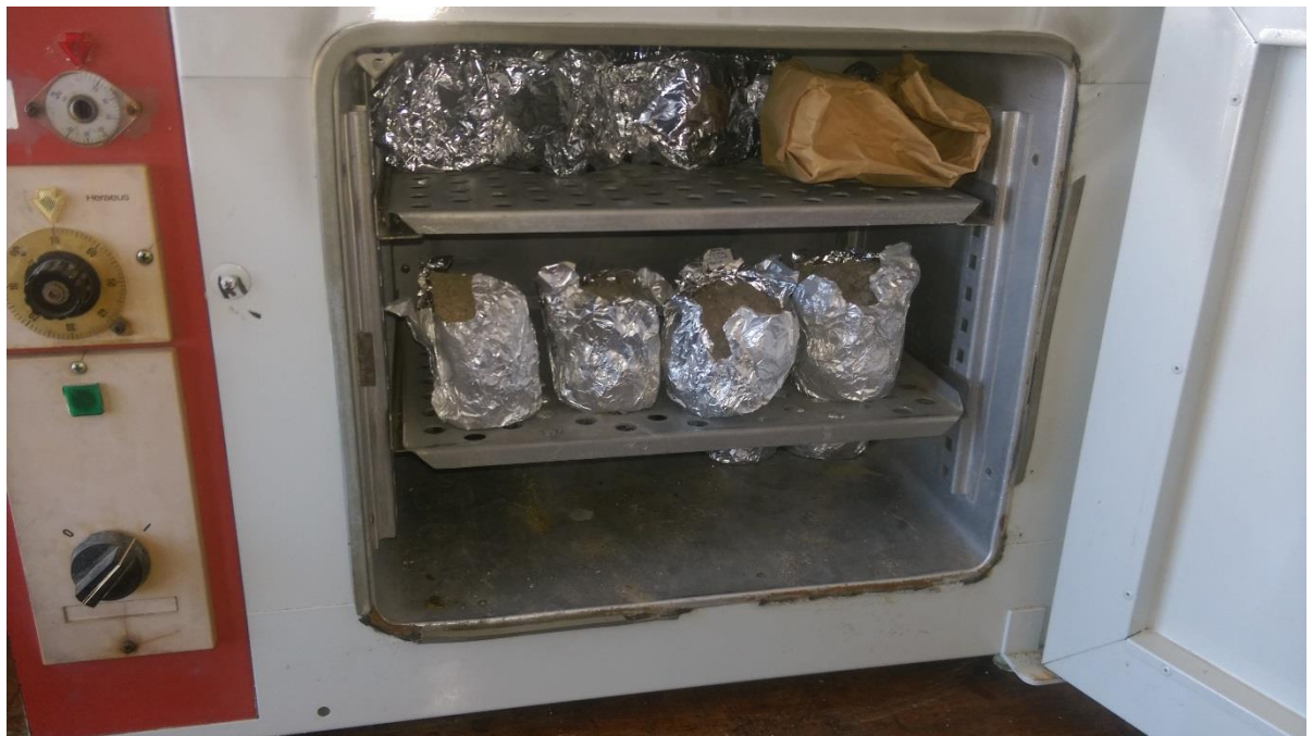
Kiln to determine organic content
