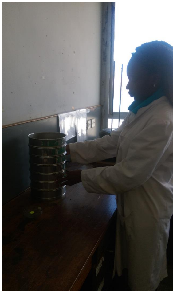
Sieves for soil texture analysis
