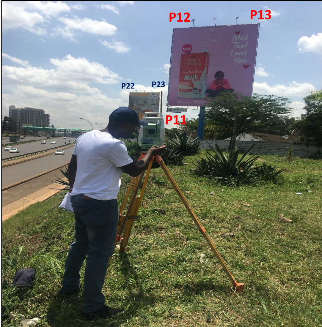
Figure 3. 3: Billboard measurements being taken using a total station
