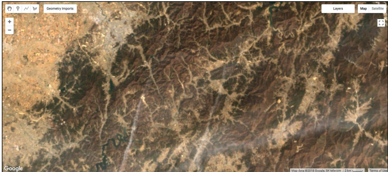
Figure 3: Landsat image corrected for SLC failure
