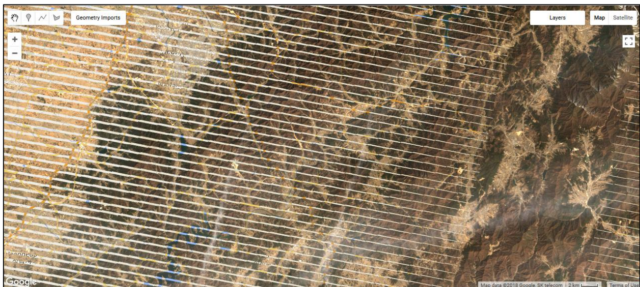
Figure 2: Landsat image with SLC failure
