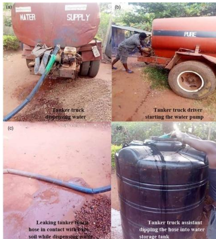
Figure 16: Undermining of informal water quality through poor handling (Source: Nnaji et al., 2019)
