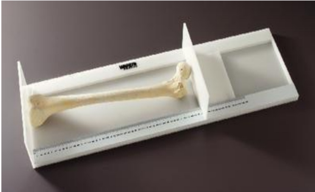
Figure 5. An osteometric board 17 used to measure the overall length of the femur.
