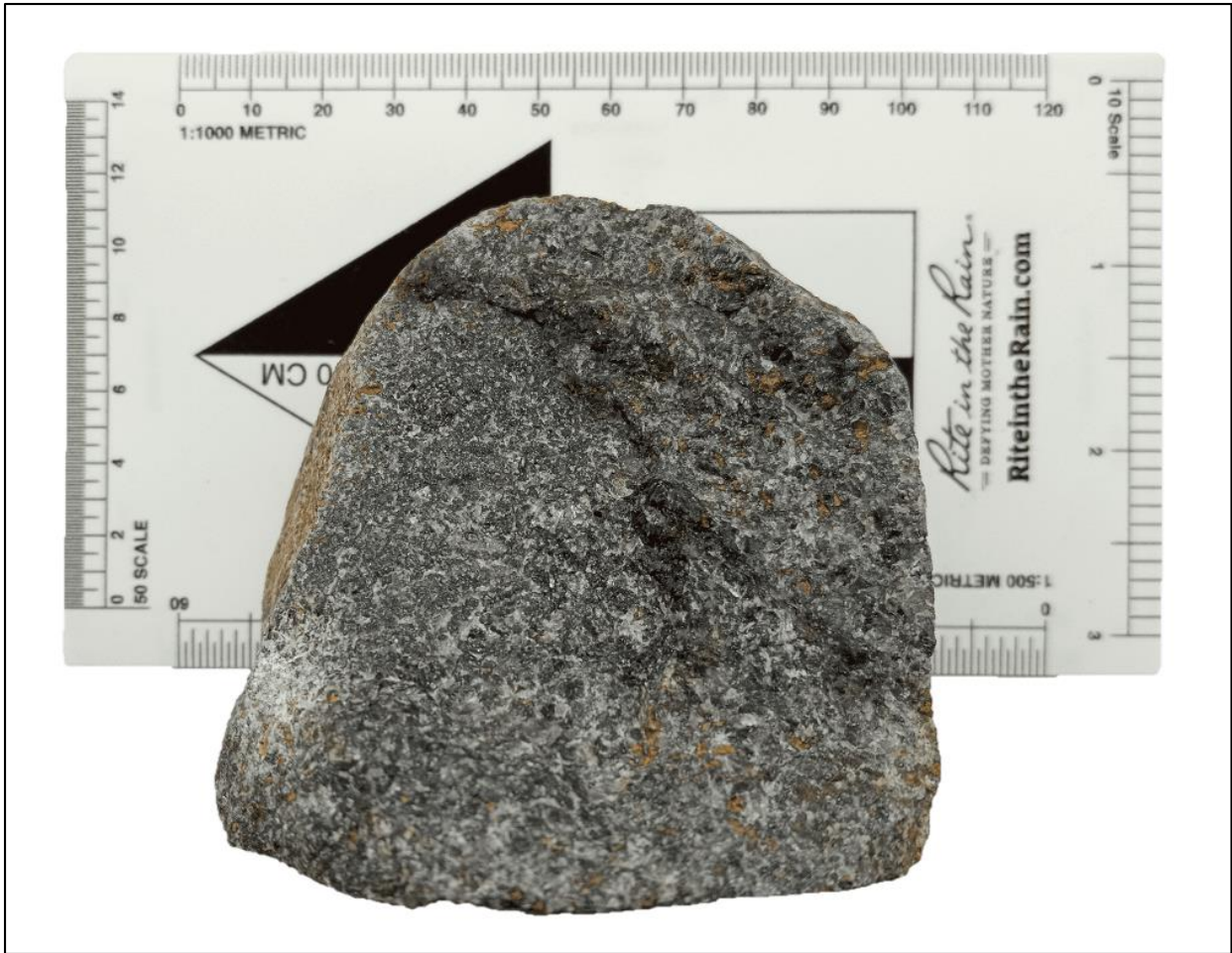
Figure 4.5: Hand specimen of sample 15 of gabbro at SMP-15 at coordinate: 0^{\circ}10'34.40''\text{S} | 37^{\circ}56'43.00''\text{E} .
