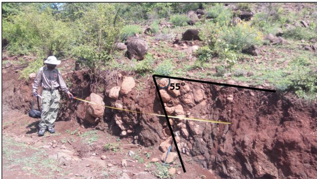
Figure 4.90: SMP-10 - 3 meter wide anorthositic gabbro boulders of centimeter-sized diameter have been fractured and dipped
