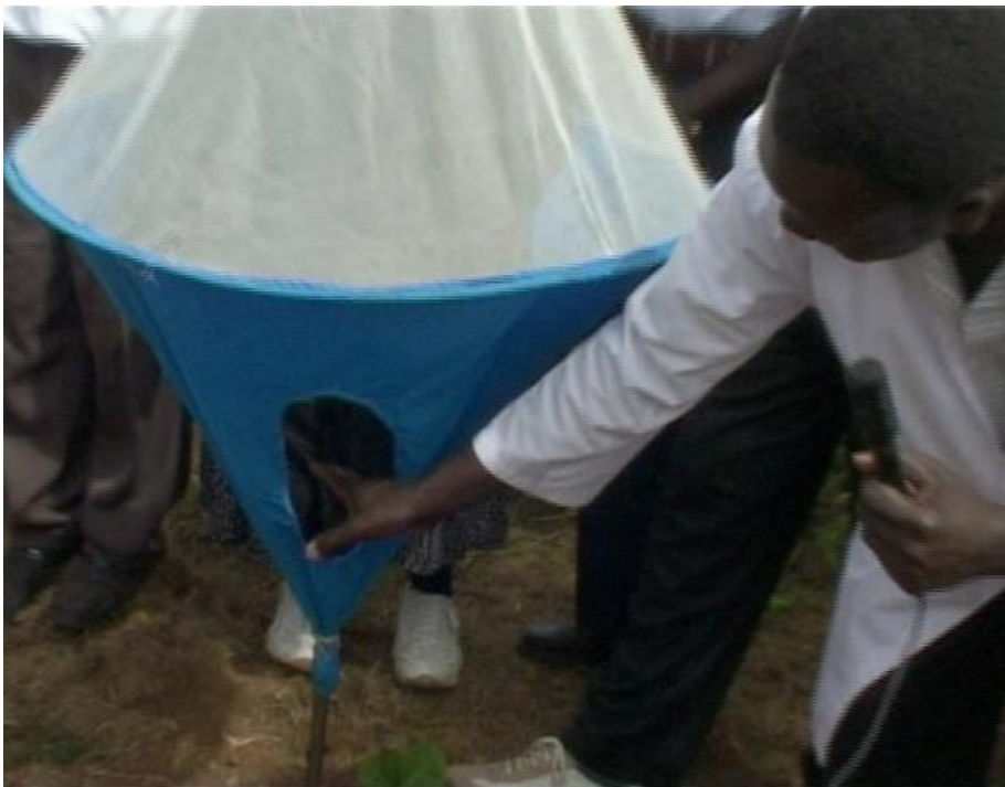
Figure 2.4: A tsetse trap used for monitoring tsetse fly populations
