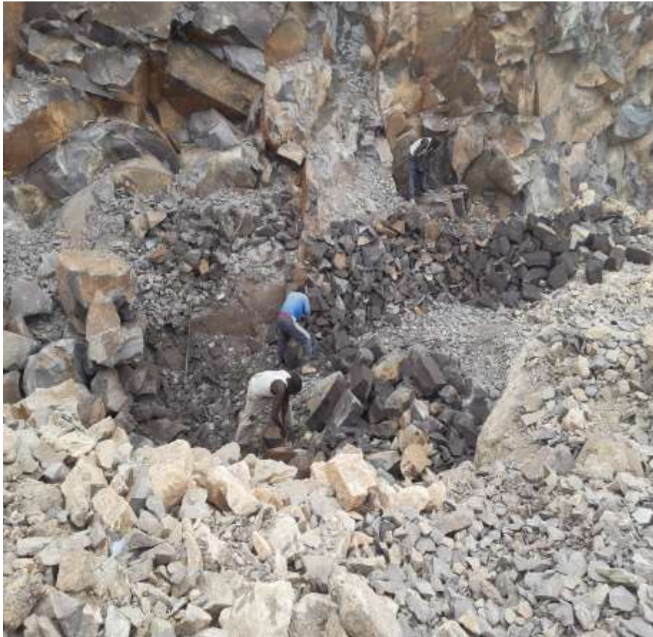
Plate 4.1: Quarry Operators without PPEs
