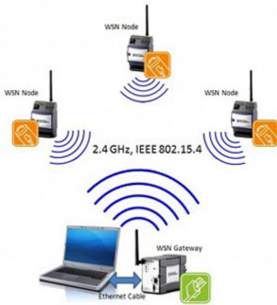
Figure 1. A Simple Wireless Sensor Network showing three sensor nodes, and a gateway connected to a laptop using a wired connection. The sensor nodes and gateway communicate wirelessly.
