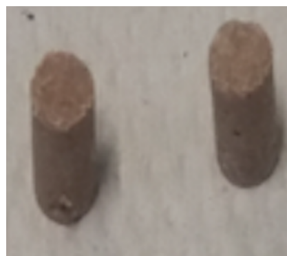
Fig 2: Kaolin-based dental cement cylinders for compressive strength tests
