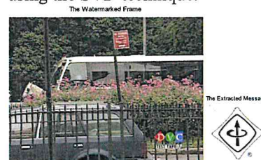
Fig 4.2: The watermarked frame at a PSNR of 50.93dB and the extracted watermark at SSIM of 0.99
