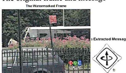
The Watermarked frame and the extracted message PSNR with 37dB and SSIM of 0.98
