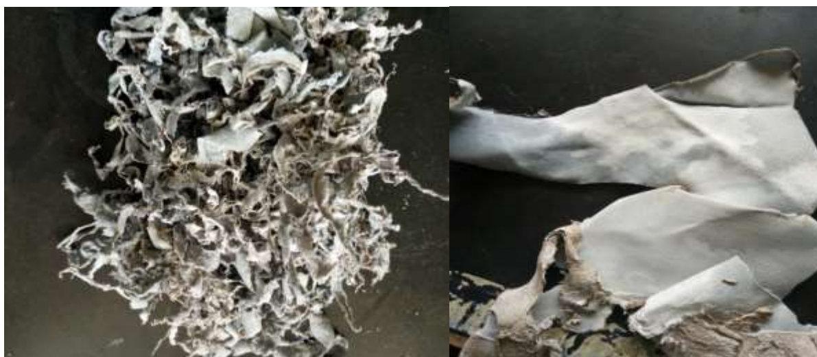
Figure 5: Chromium tanned trimmings obtained from tanned leather.
