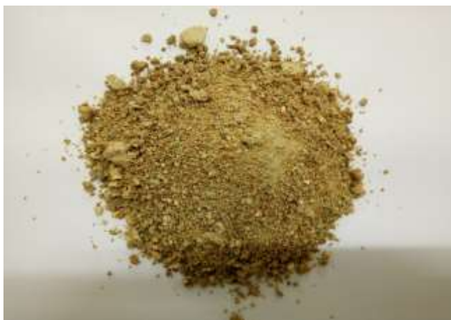
Figure 11: Freeze dried powder obtained from the gelatin solution
