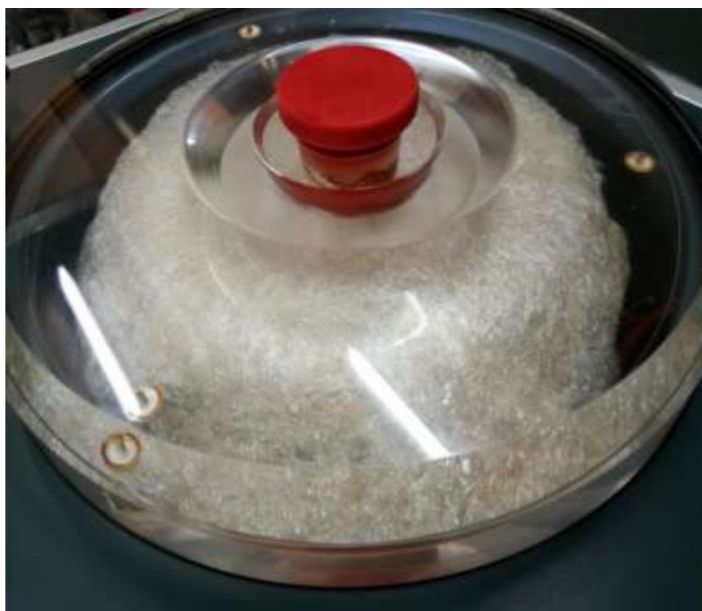
Figure 7: Freeze drying of gelatin obtained from hydrolysis of leather trimmings
