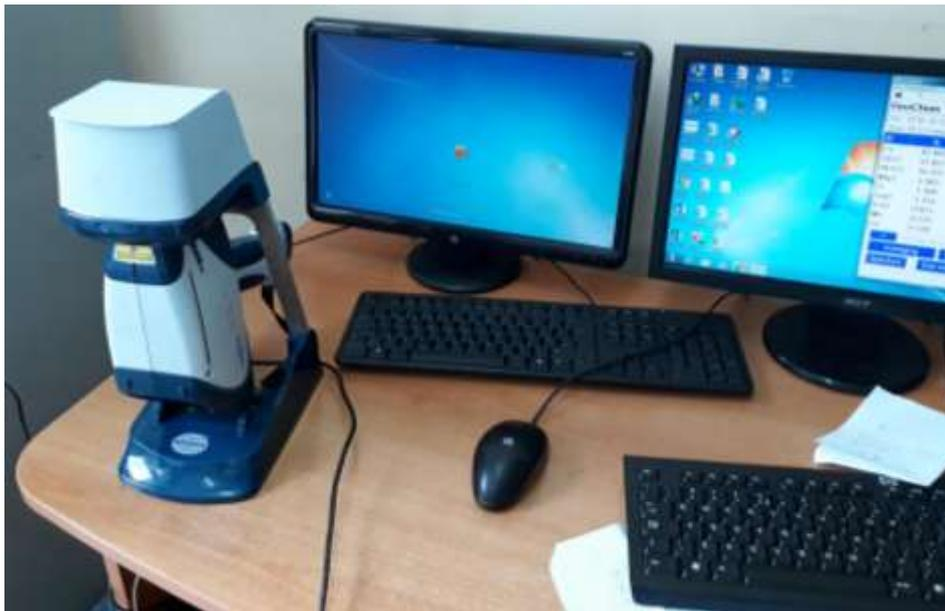
**Figure 3.10: Portable XRF Analyzer (BRUKER S1 TITAN 800).**
