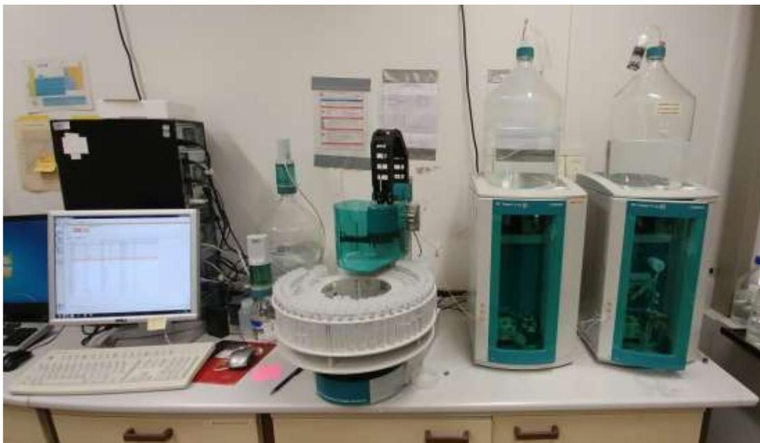
**Figure 3.6: Ion chromatography instrument (Metrohm system: 881 Compact IC pro – Anion, Cation).**
