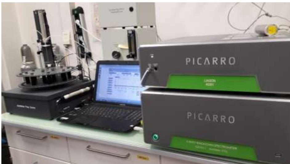
**Figure 3.4: Picarro cavity ring-down spectrometer (G2101-i Isotopic  $\text{CO}_2$ ).**
