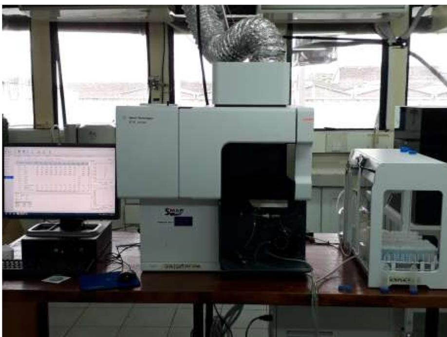
**Figure 3.8: ICP-OES instrument (Agilent Technologies 5110).**
