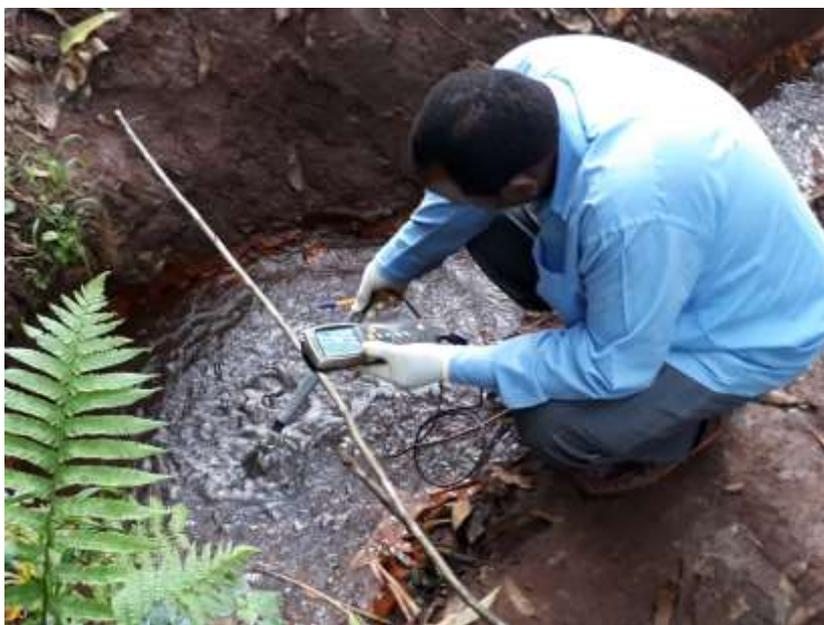
**Figure 3.2: Measurement of ambient CO<sub>2</sub> at Mbwinjeru spring using NDIR CO<sub>2</sub> Sensor (Testo 435).**
