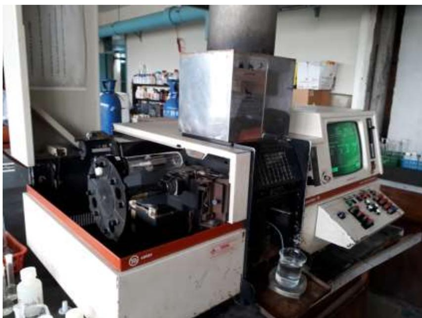
**Figure 3.9: AAS instrument (VARIAN SPECTRA A-10).**
