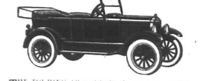
THE TOURING All-steel body of stream-line design. Double ventilating windshield (one-piece) high top hood under front seat. Standard equipment includes cord tires, new type tyre carrier, wiper, proof ash curtains opening with all doors, hood cover, windshield wiper, nickel plated radiator shell and headlamp rims.
