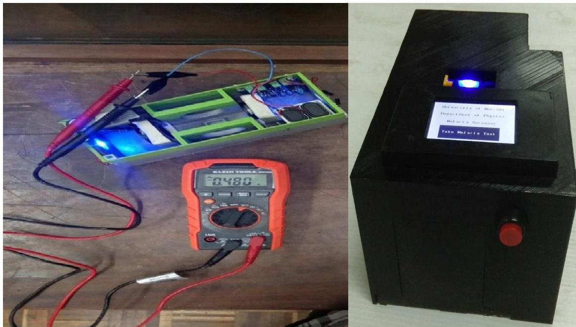
Figure 4.11: The low cost malaria screening device
