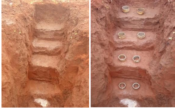
Figure 5. Profile pit with core rings collecting undisturbed soil samples in Katumani
