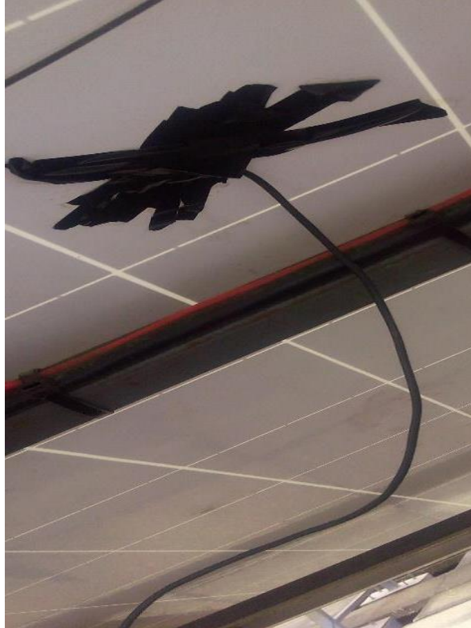
Figure 4.3: Temperature sensor PT300N attached with adhesive tape at the back of a solar module.
