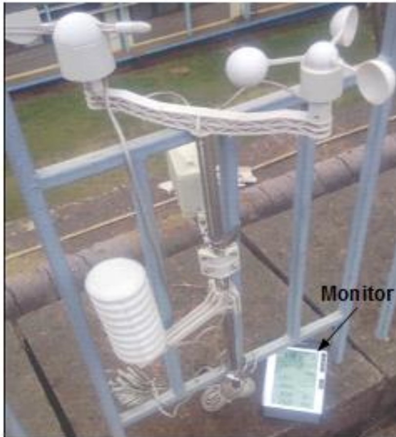
Figure 4.6: A picture of the portable Weather station installed at the School of Physical sciences, University of Nairobi the radio-controlled monitor displaying real time weather data is also shown.
