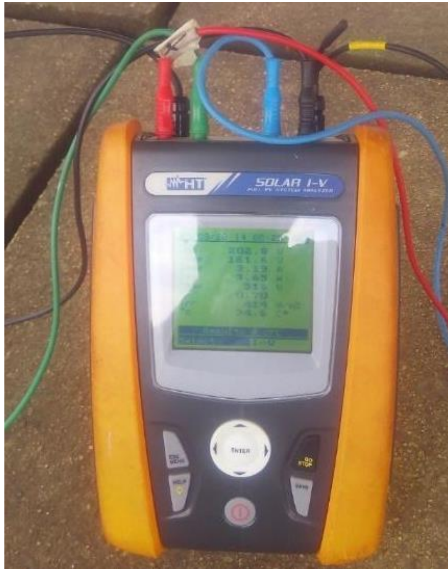
Figure 4.4: Solar Current –Voltage (I-V) 400 analyzer from HT instruments.
